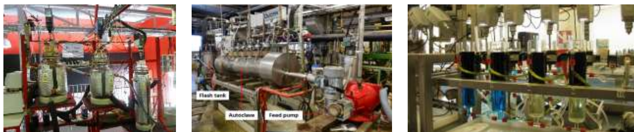
FIGURE 2. TR LEAD AND SILVER LEACHING PILOT PLANT (LEFT). OUTOTEC LEAD PRESSURE LEACHING PILOT PLANT (CENTRE).OUTOTEC Cu SX PILOT PLANT MIXER SETTLERS (RIGHT).
