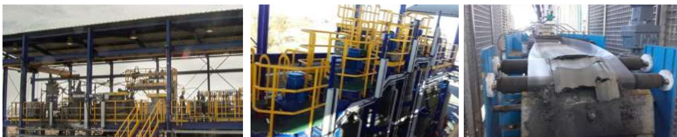
FIGURE 1. CLC FLOTATION PILOT PLANT (LEFT). CLC ATMOSPHERIC LEACHING PILOT PLANT: REACTORS CASCADE AND FILTRATION (RIGHT).
