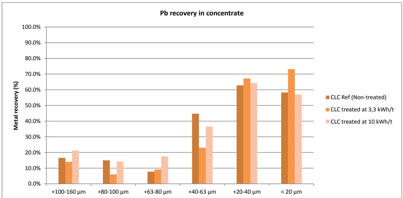
FIGURE 88 - PB RECOVERY PER SIZE FRACTION IN FLOTATION CONCENTRATE OF CLC TREATED AND UNTREATED SAMPLES.
