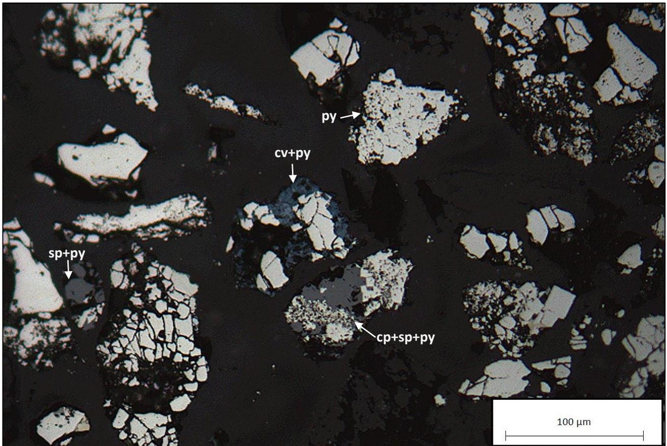
FIGURE 73 - PICTURES OF LIGHT TRANSMITTED MICROSCOPE OBSERVATION OF A 100-160 MICRONS FRACTION FROM A GROUND CLC SAMPLE.
