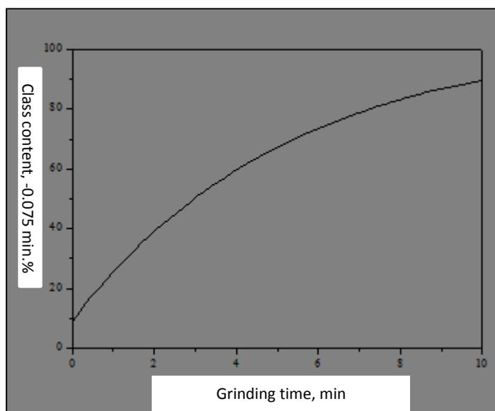
FIGURE 65 - DEPENDANCE THE CLASS CONTENT -0,075MM ON GRINDING TIME.
