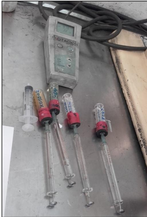
FIGURE 36 - REAGENTS ADDITION IN LAB FLOTATION TESTS.
