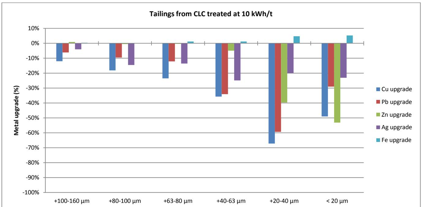
FIGURE 86 - METAL UPGRADE WITHIN TAILINGS THE FLOTATION TRIAL FROM CLC MICROWAVE TREATED SAMPLE AT 10 KWH/T.
