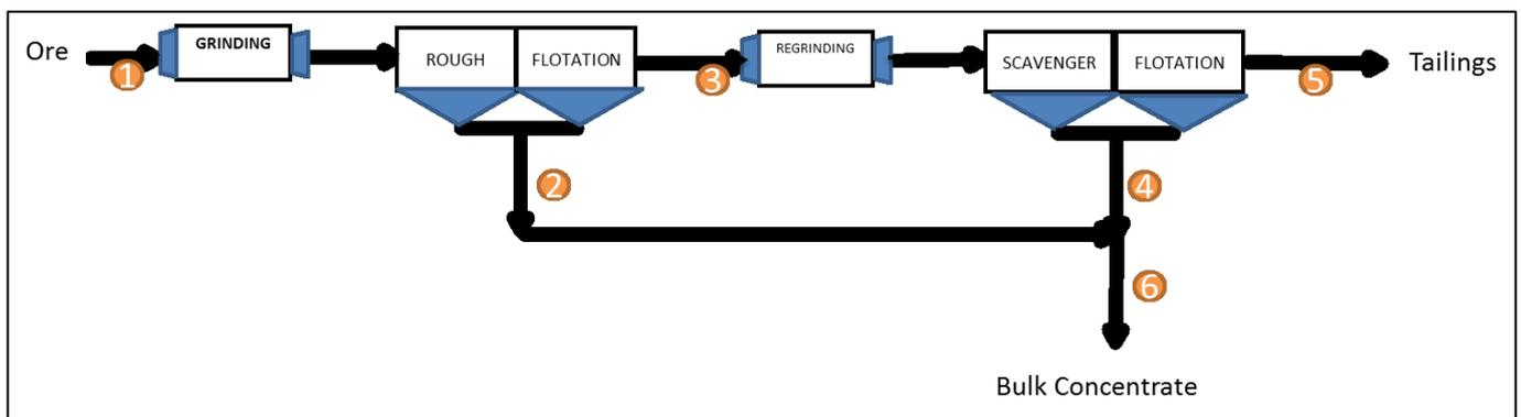
FIGURE 47. FLOTATION SCHEME.
