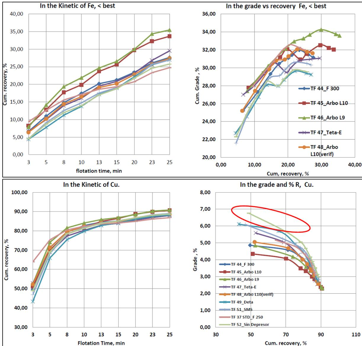
FIGURE 45. EFFECT OF PYRITE DEPRESSANTS.
