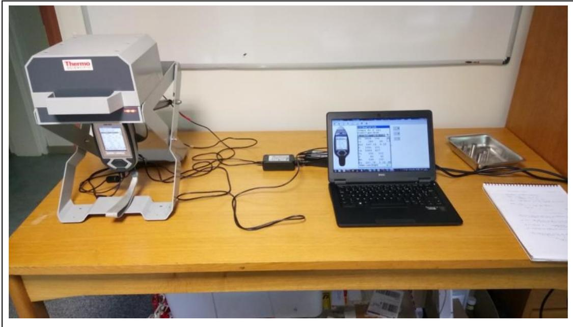
**FIGURE 79 - FPXRF STATION USED TO PERFORM METALLURGICAL ASSAYS OF FLOTATION TRIALS PRODUCTS.**
