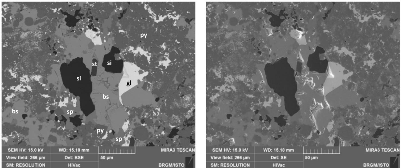
**FIGURE 25 - BSE (LEFT) AND SE (RIGHT) PICTURES OF A BOR SAMPLE MICROWAVE TREATED AT 10 KWH/T (BS: BARUYM SULFATE; SP: SPHALERITE; SI: SILICA; ST: SILICATE; GL: GALENA; PY: PYRITE).**
