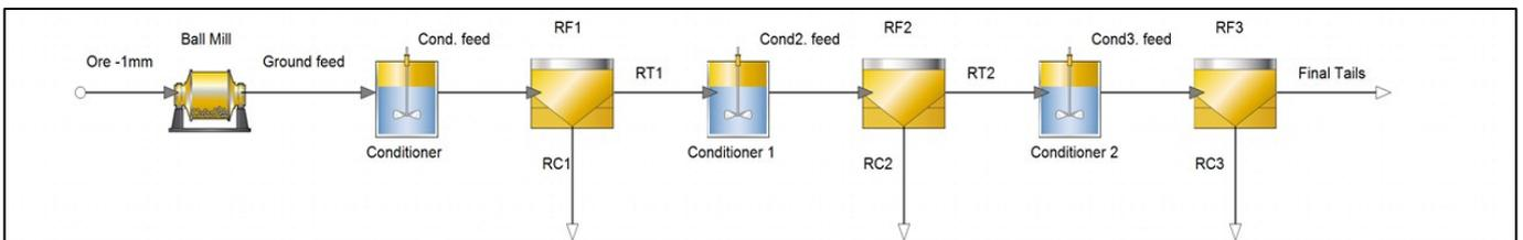
FIGURE 54 - PROCESS FLOW SHEET FOR SEQUENTIAL FLOTATION.
