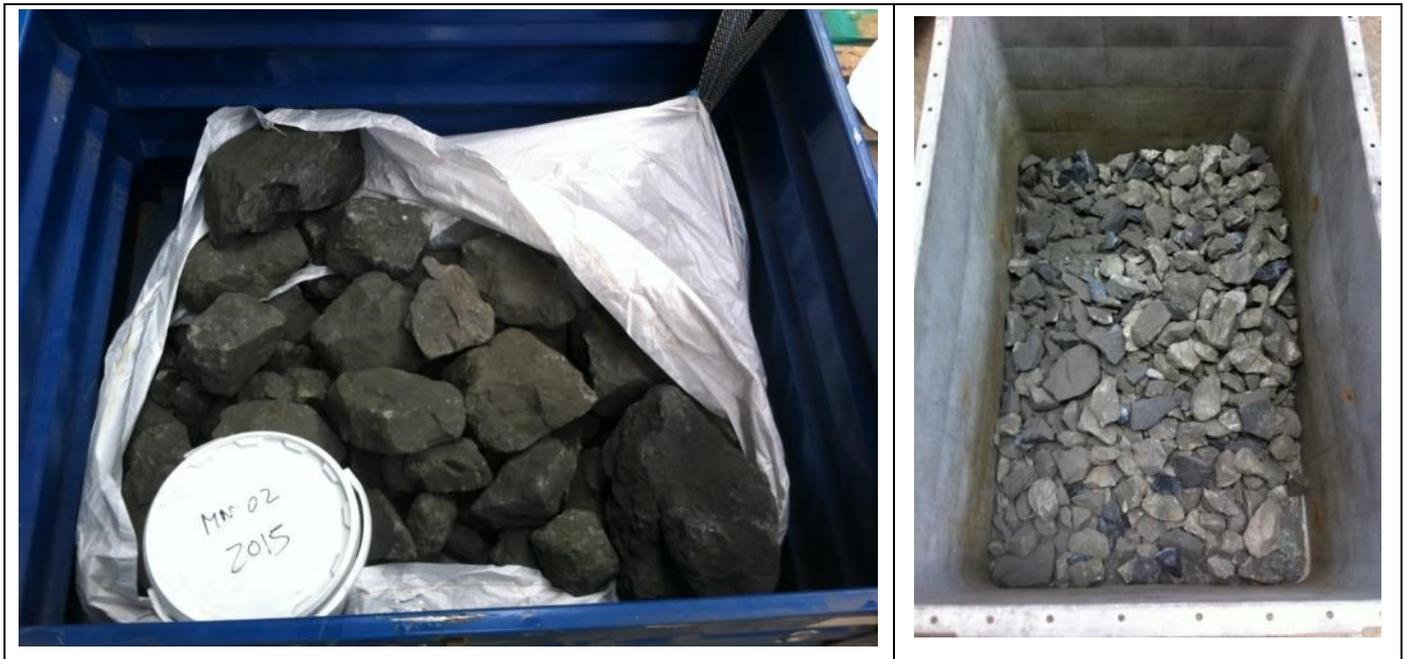
**FIGURE 5 - COBRE LAS CRUCES RUN OF MINE ORE AS RECEIVED AND AFTER JAW CRUSHER.**
