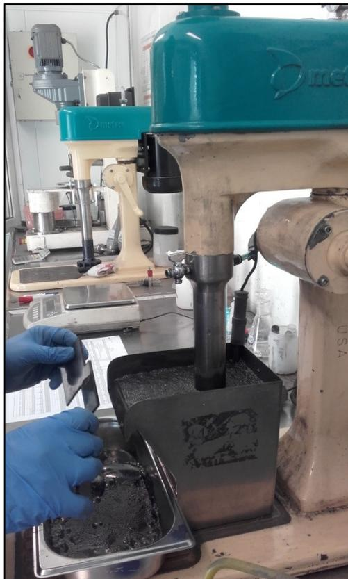
FIGURE 38 - LAB FLOTATION CELL.
