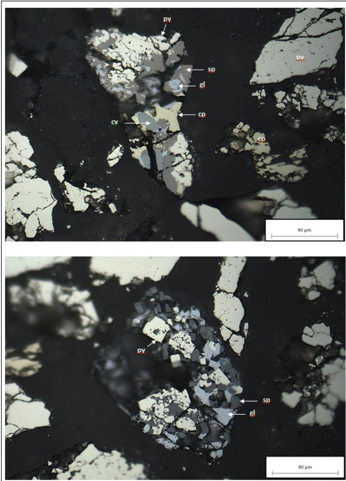
FIGURE 74 - PICTURES OF LIGHT TRANSMITTED MICROSCOPE OBSERVATION OF A 63-80 MICRONS FRACTION FROM A GROUND CLC SAMPLE.
