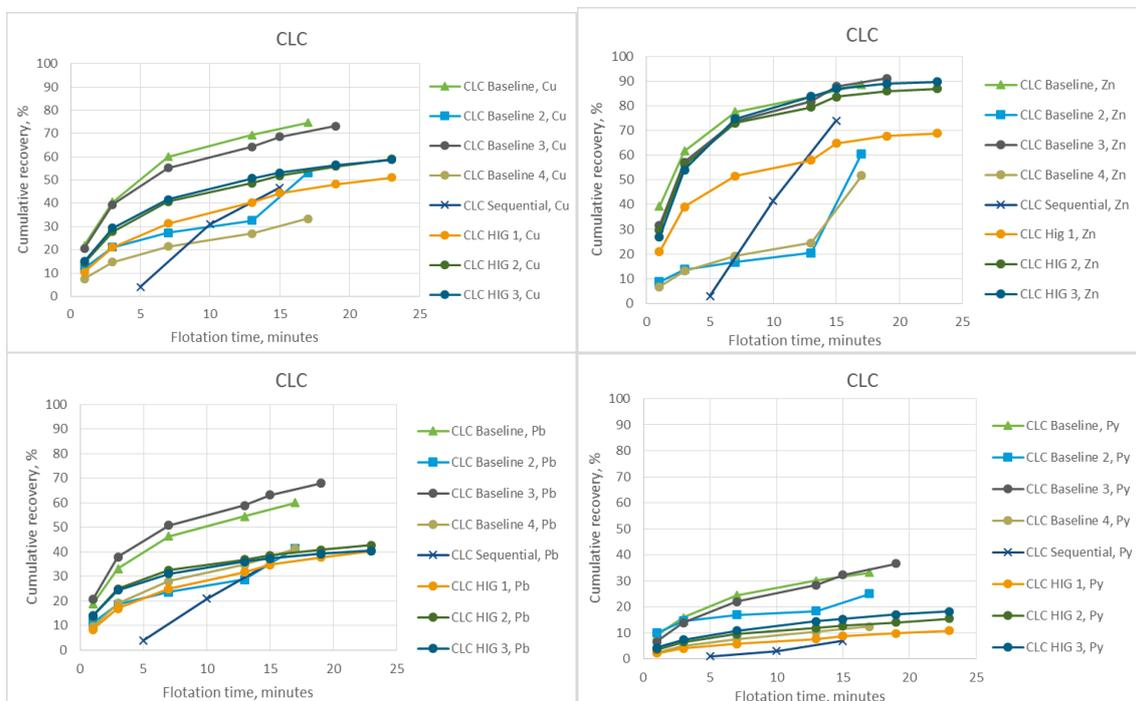
FIGURE 57 - CUMULATIVE RECOVERIES FOR COPPER, ZINC, LEAD AND PYRITE FOR THE FLOTATION TESTS WITH CLC ORE.
