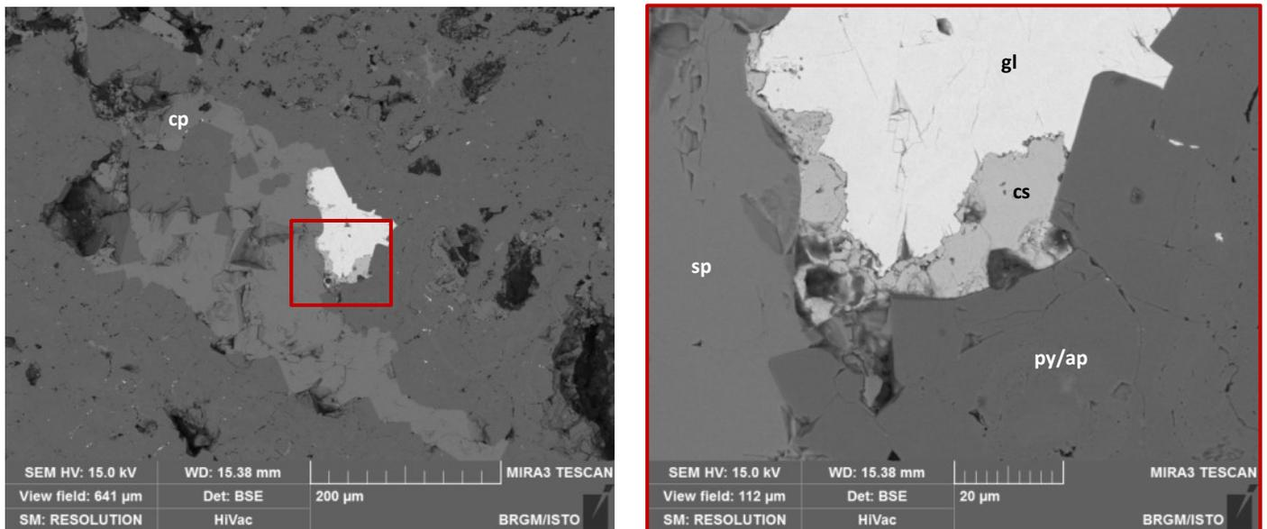
**FIGURE 20 - BSE PICTURES OF A CLC ORE SAMPLE TREATED AT 30 KWH/T (GL: GALENA; SP: SPHALERITE; PY: PYRITE; CP: CHALCOPYRITE; AP: ARSENOPYRITE; CS: CERUSSITE).**
