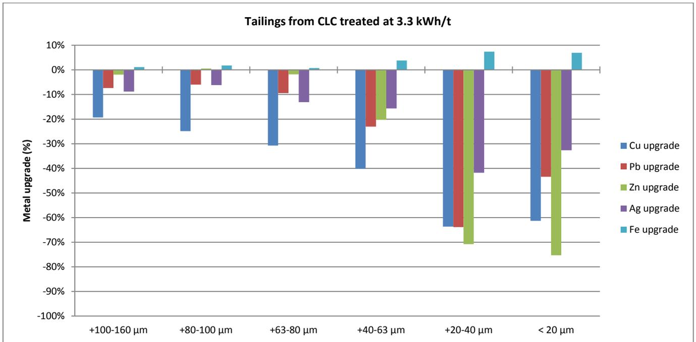
FIGURE 85 - METAL UPGRADE WITHIN TAILINGS OF FLOTATION TRIAL FROM CLC MICROWAVE TREATED SAMPLE AT 3.3 KWH/T.
