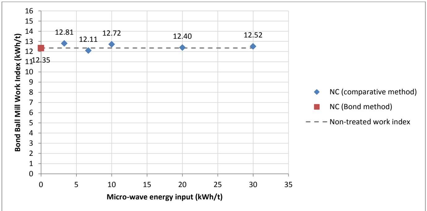
FIGURE 27 - BOND BALL MILL WORK INDEX OF NC MICROWAVE TREATED AND UNTREATED SAMPLES.
