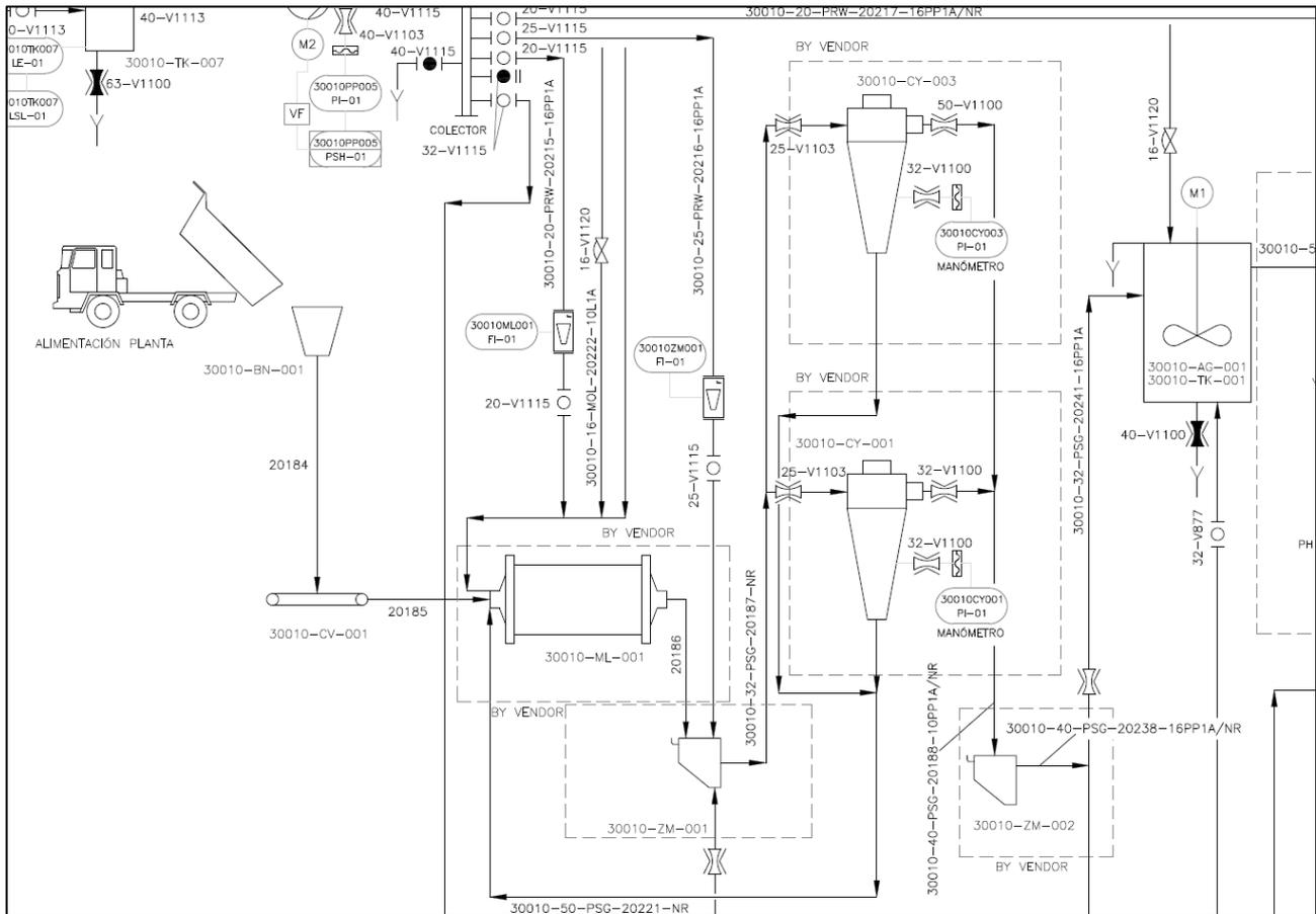
FIGURE 107 - P&ID VIEW OF GRINDING STAGE.
