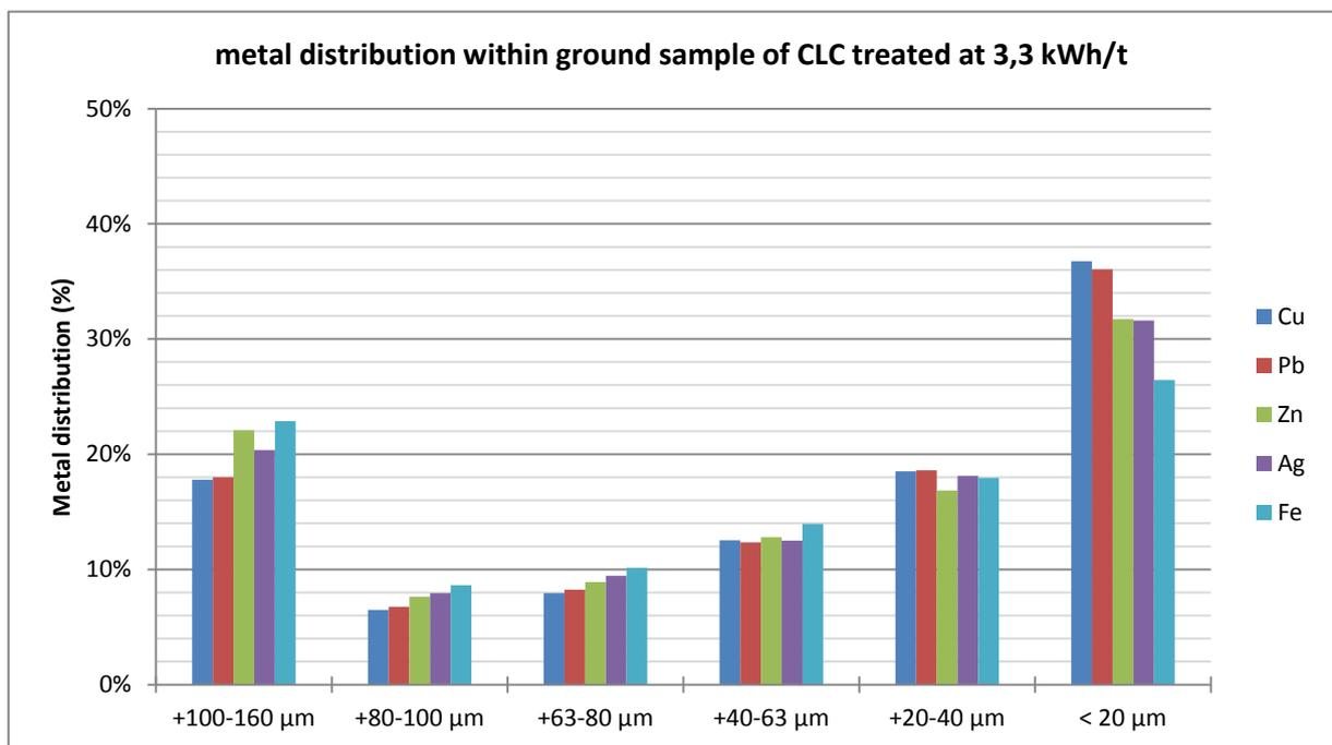
FIGURE 82 - METAL DISTRIBUTIONS BY SIZE FRACTION WITHIN GROUND SAMPLE OF CLC TREATED AT 3.3 KWH/T.
