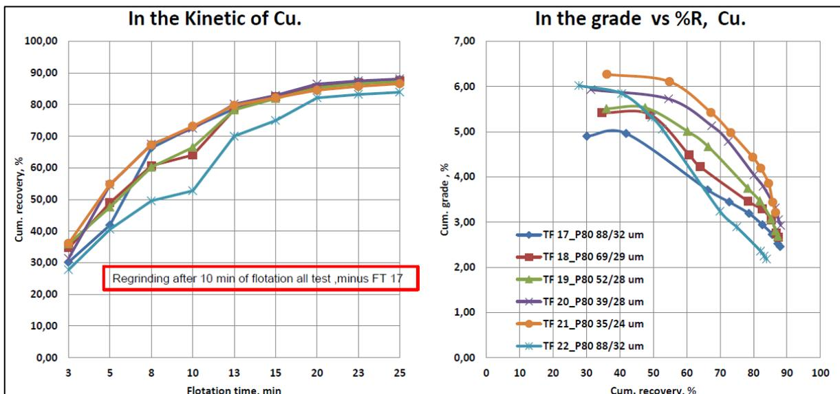
FIGURE 42 - COPPER KINETIC, GRADE AND RECOVERY VS PARTICLE SIZE.
