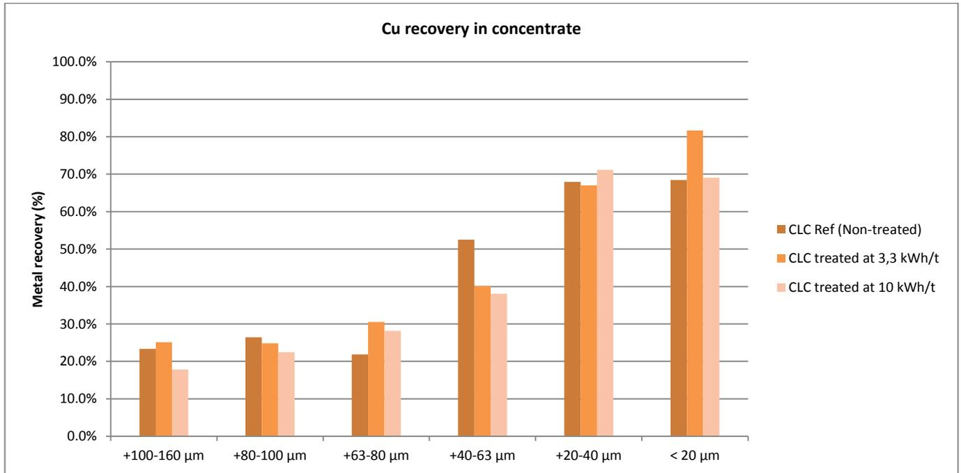
FIGURE 87 - CU RECOVERY PER SIZE FRACTION IN FLOTATION CONCENTRATE OF CLC TREATED AND UNTREATED SAMPLES.
