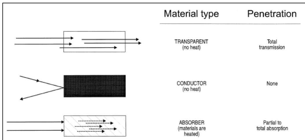
FIGURE 1 - INTERACTION OF MICROWAVE WITH MATERIALS (FROM HAQUE, 1999).
