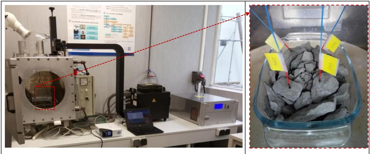
**FIGURE 10 - [LEFT] EXPERIMENTAL SET-UP OF WITH THE MICROWAVE OVEN, THE MAGNETRON, THE GENERATOR, AND THE THERMOMETER; [RIGHT] CLOSE LOOK AT THE FIBER OPTIC TEMPERATURE SENSOR WITHIN CARVED HOLES FOR TEMPERATURE MONITORING.**
