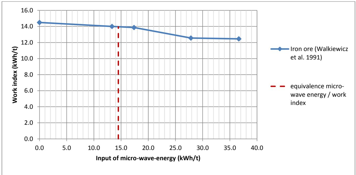
FIGURE 2 - EVOLUTION OF THE WORK INDEX OF IRON ORE SAMPLES WITH INCREASING INPUT MICRO-WAVE ENERGY (WALKIEWICZ ET AL. 1991).
