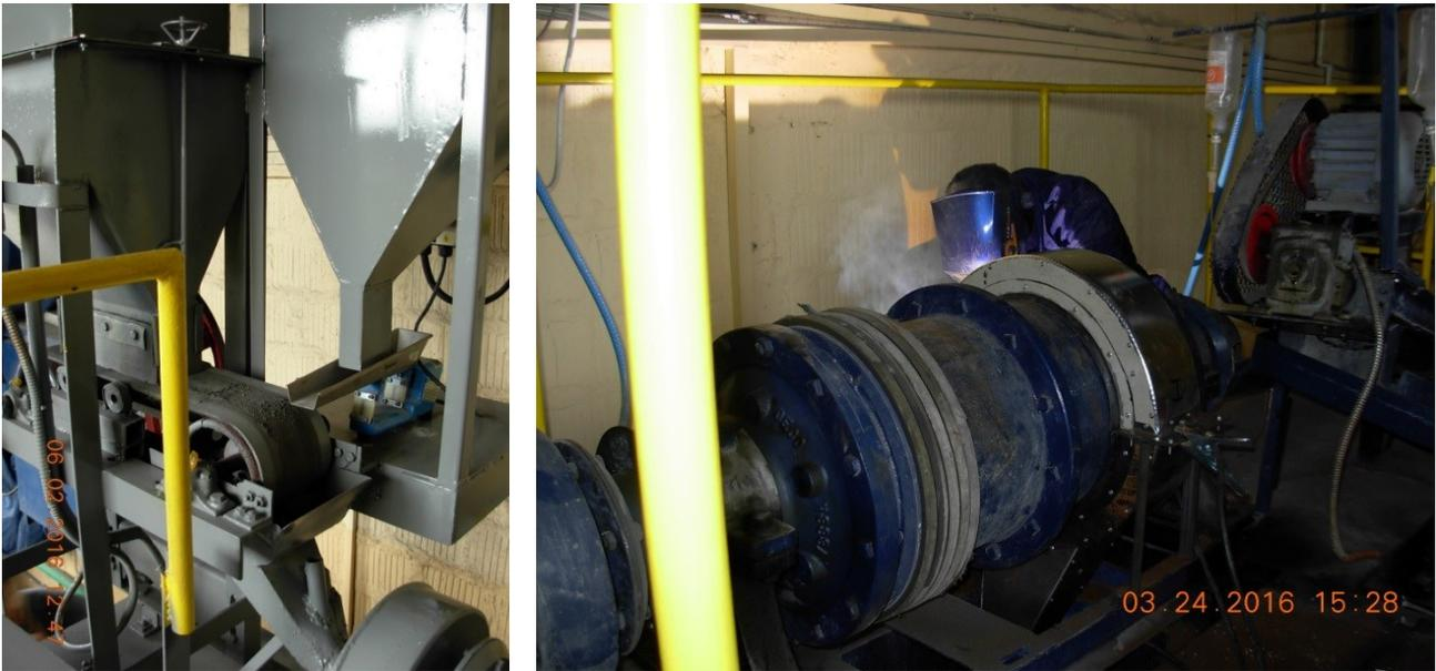
**FIGURE 92 – LEFT: BINS AND FEEDERS FOR ORE AND LIME; RIGHT: MILL RECONSTRUCTION.**
