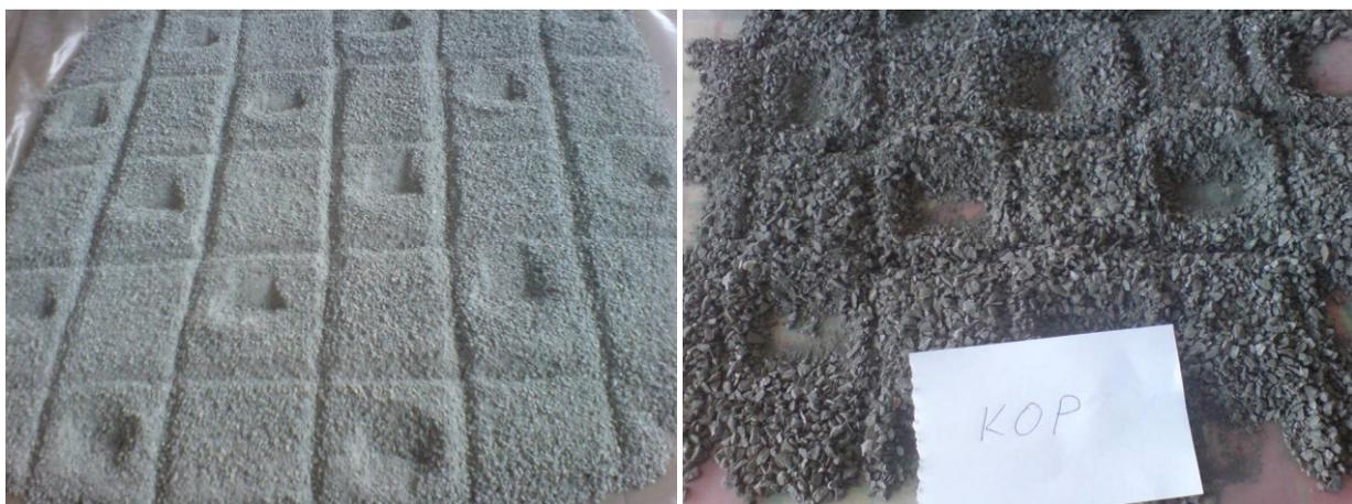
FIGURE 63 - SAMPLING TECHNOLOGY TEST. SAMPLING FOR MINERALOGICAL ANALYSIS.
