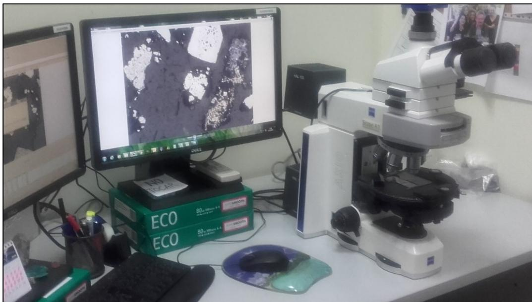
FIGURE 33 - METALLOGRAPHIC MICROSCOPE.
