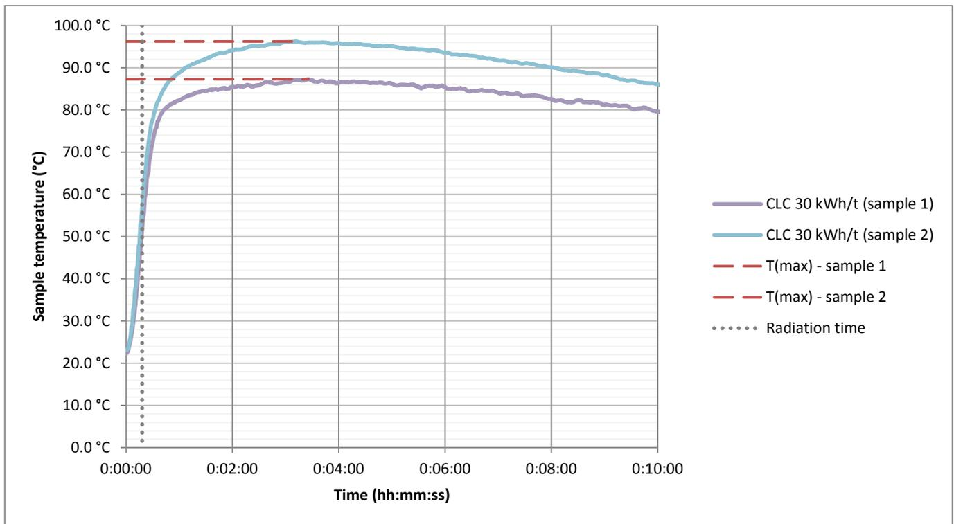
FIGURE 13 – TEMPERATURE MONITORING CLC SAMPLES MICRO-WAVE TREATED AT 30 KWH/T (RADIATION TIME: 18 SEC).
