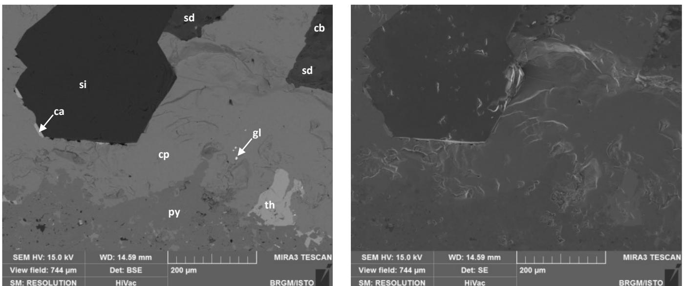
**FIGURE 24 – BSE (LEFT) AND SE (RIGHT) PICTURES OF A NC ORE SAMPLE TREATED AT 10 KWH/T (CP: CHALCOPYRITE; TH: TETRAHEDRITE; PY: PYRITE; GL: GALENA; SI: SILICA; SD: SIDERITE; CB: CARBONATE CA/MG; CA: CASSITERITE).**
