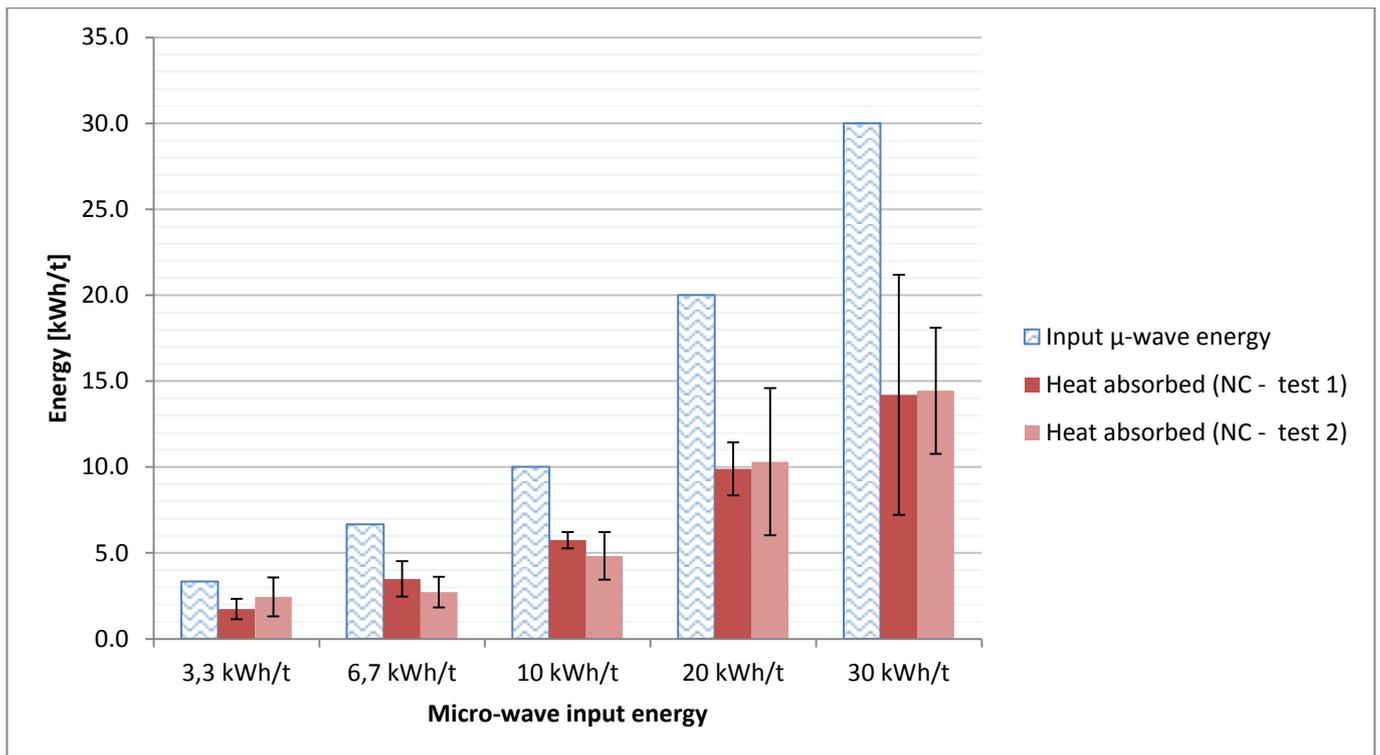
FIGURE 16 - CHART OF INPUT MICROWAVE ENERGY AND HEAT ABSORBED BY NC SAMPLES.
