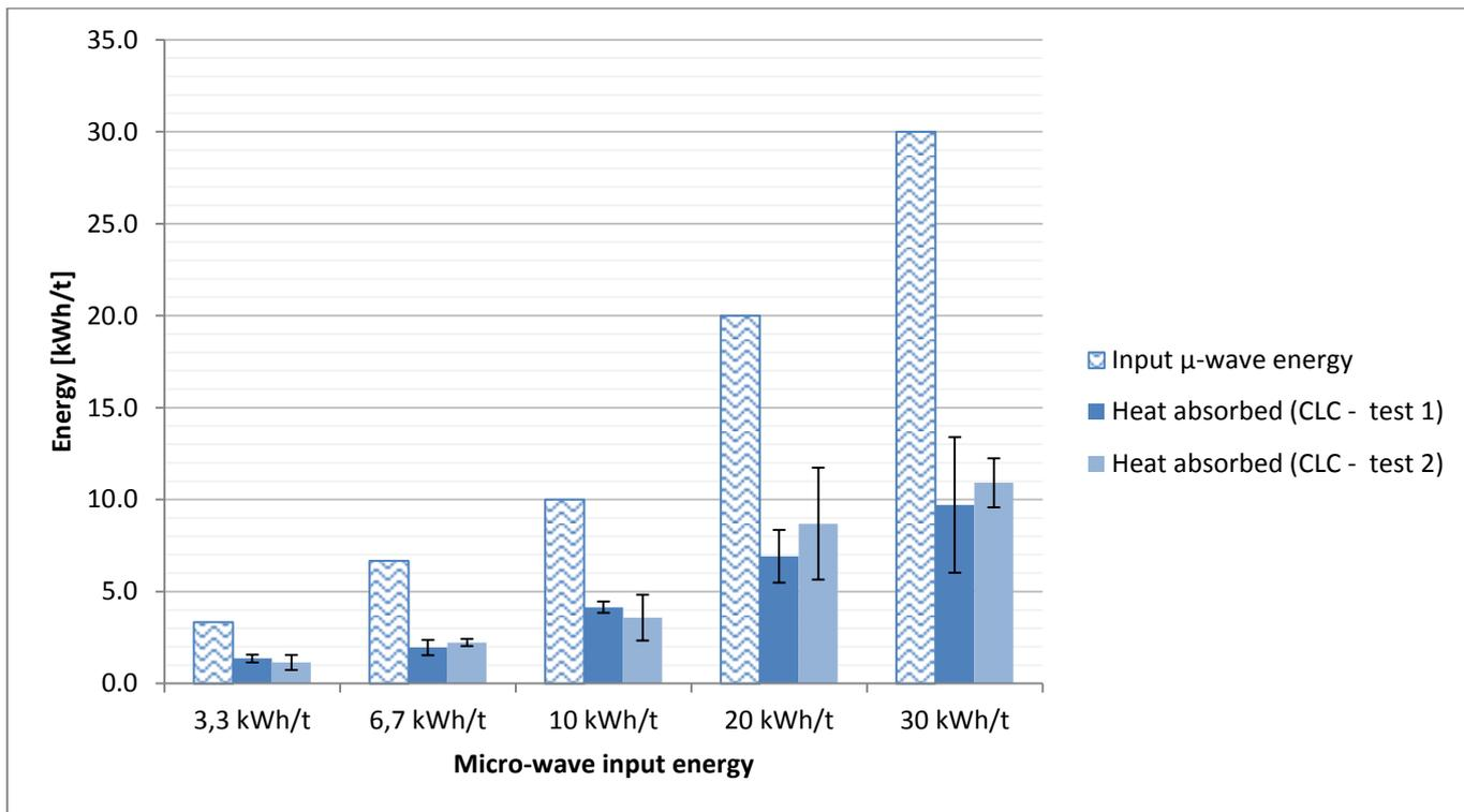
FIGURE 14 - CHART OF INPUT MICROWAVE ENERGY AND HEAT ABSORBED BY CLC SAMPLES.
