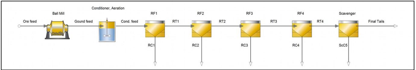
FIGURE 53 - PROCESS FLOW SHEET FOR BULK FLOTATION.
