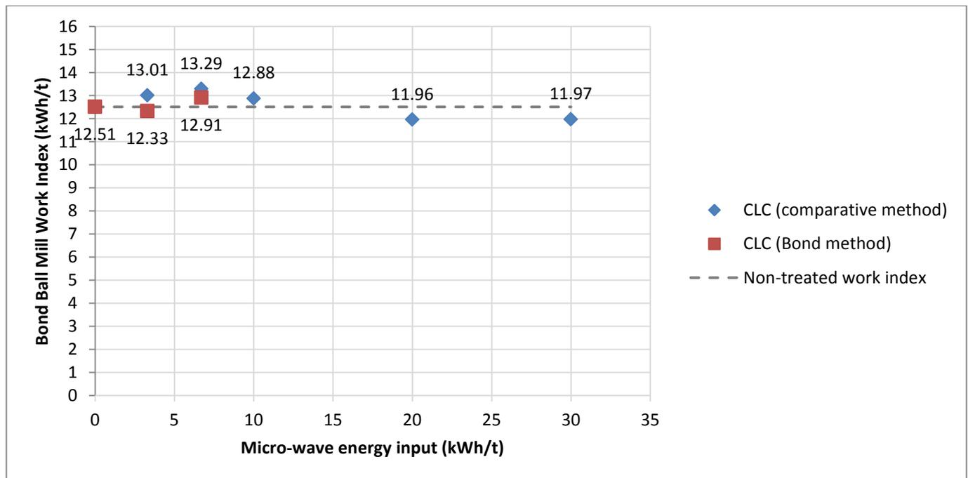
FIGURE 26 – BOND BALL MILL WORK INDEX OF CLC MICROWAVE TREATED AND UNTREATED SAMPLES.
