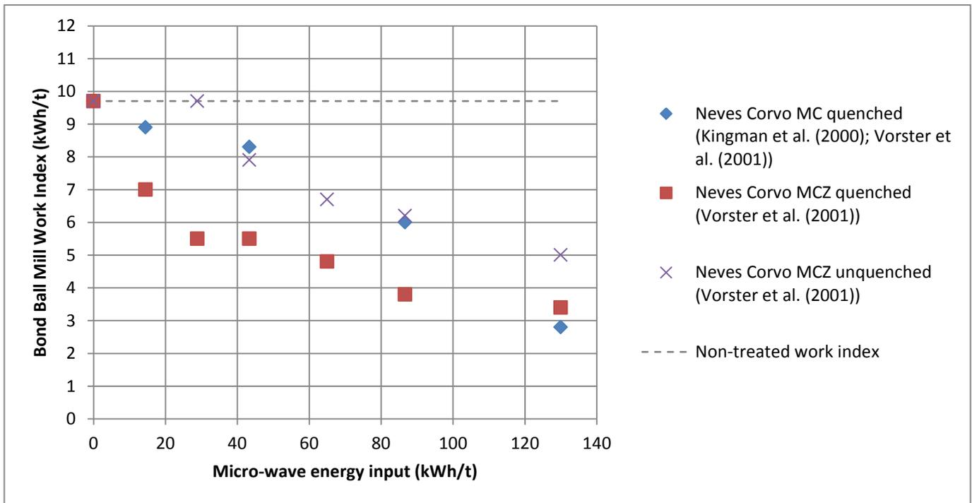
FIGURE 4 - EXPERIMENTAL RESULTS ADAPTED FROM KINGMAN ET AL. (2000) AND VORSTER ET AL. (2001) OF THE MICROWAVE TREATMENT OF NEVES CORVO MC AND MCZ ORES.
