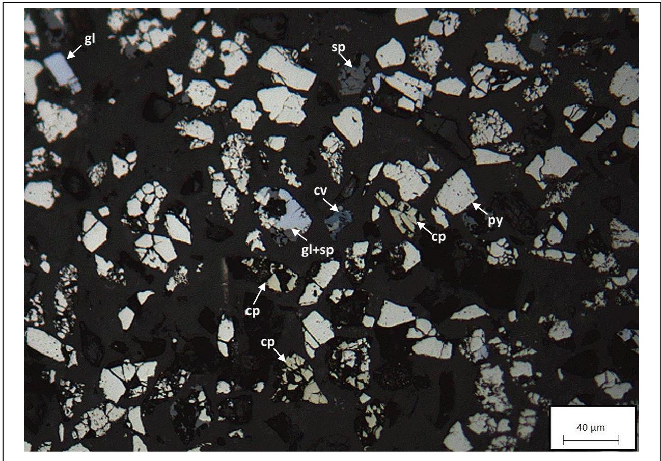
**FIGURE 75 - PICTURES OF LIGHT TRANSMITTED MICROSCOPE OBSERVATION OF A 20-40 MICRONS FRACTION FROM A GROUND CLC SAMPLE (GL: GALENA; SP: SPHALERITE; PY: PYRITE; CP: CHALCOPYRITE; CV: COVELLITE)**
