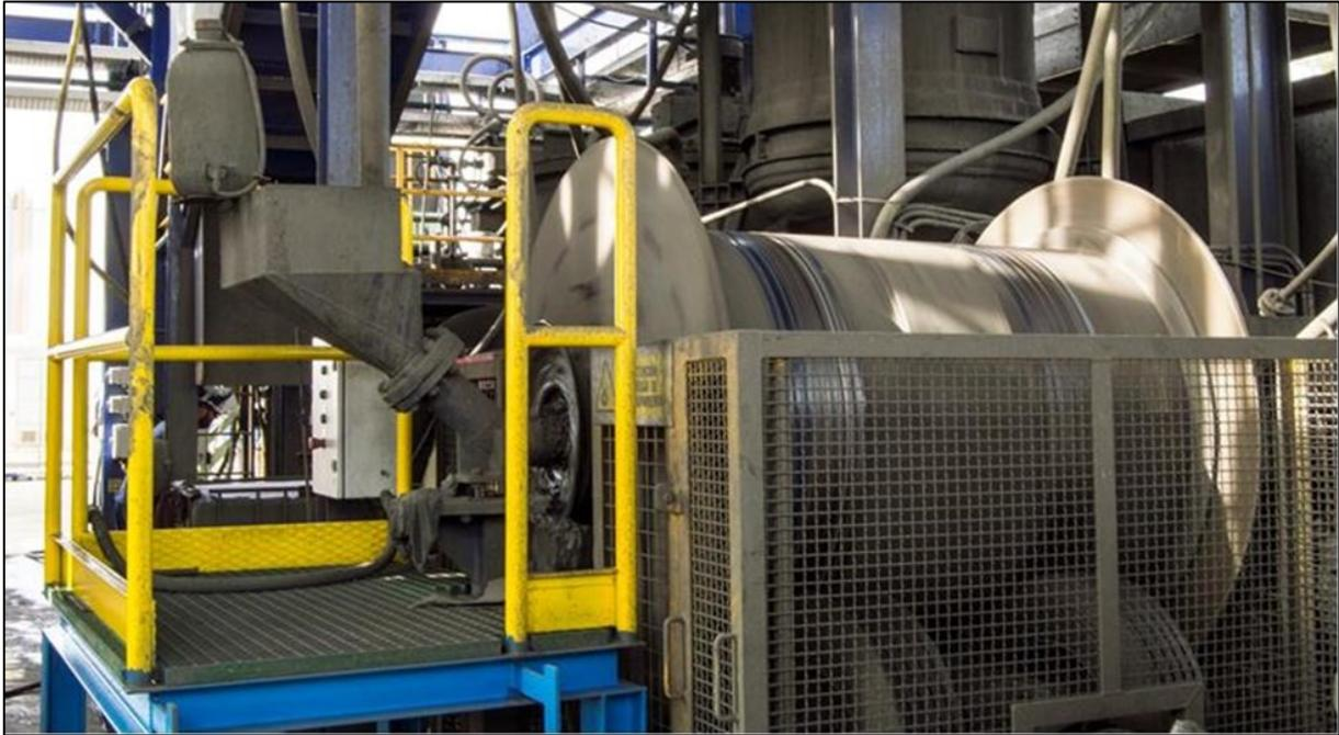
FIGURE 106 - CLC FLOTATION PILOT PLANT. REGRINDING BALL MILL.
