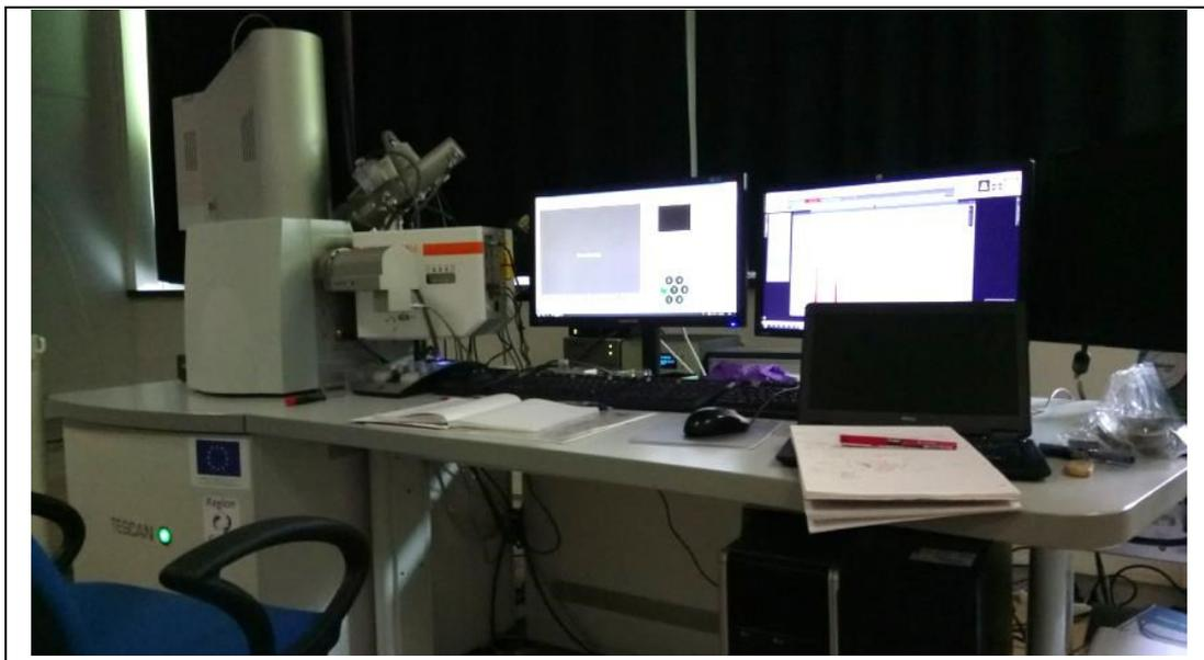
**FIGURE 11 - SCANNING ELECTRON MICROSCOPE (SEM) COUPLED WITH AN ENERGY DISPERSIVE SPECTROSCOPY (EDS).**
