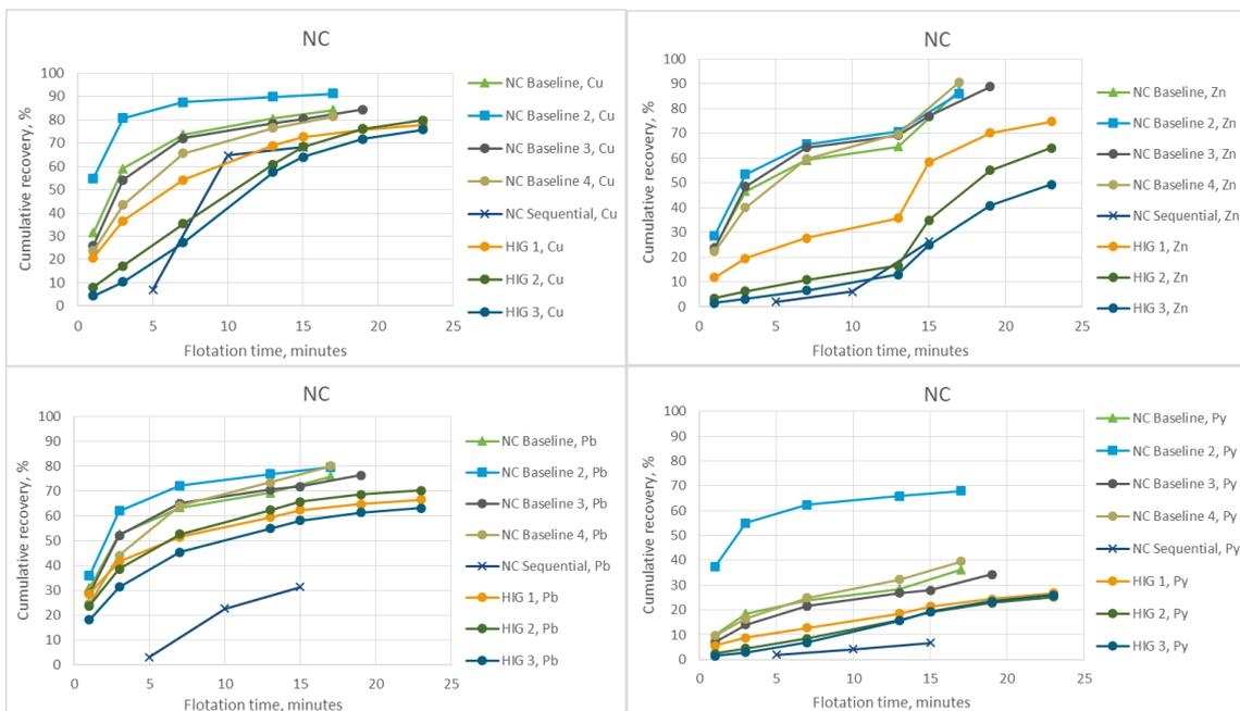
**FIGURE 56 - CUMULATIVE RECOVERIES FOR COPPER, ZINC, LEAD AND PYRITE FOR THE FLOTATION TESTS WITH NEVES CORVO ORE.**
