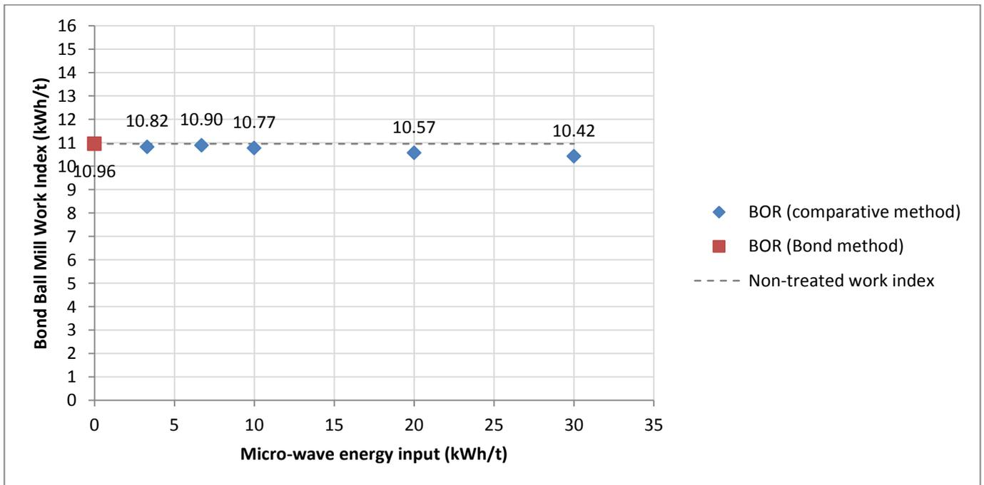
FIGURE 28 - BOND BALL MILL WORK INDEX OF BOR MICROWAVE TREATED AND UNTREATED SAMPLES.
