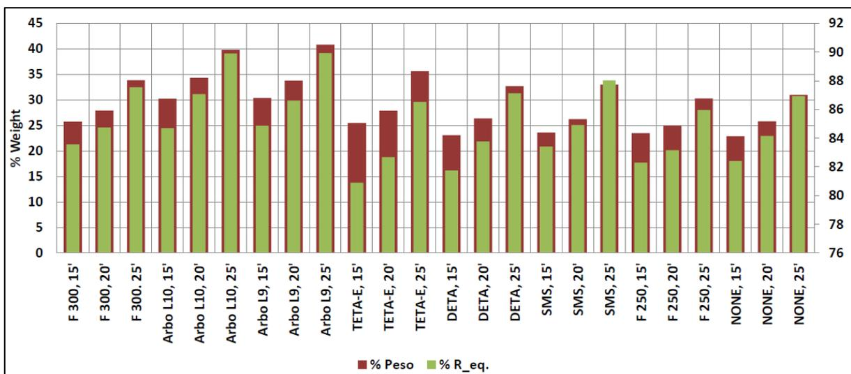
FIGURE 44 - MASS RECOVERY VS PYRITE DEPRESSANTS.
