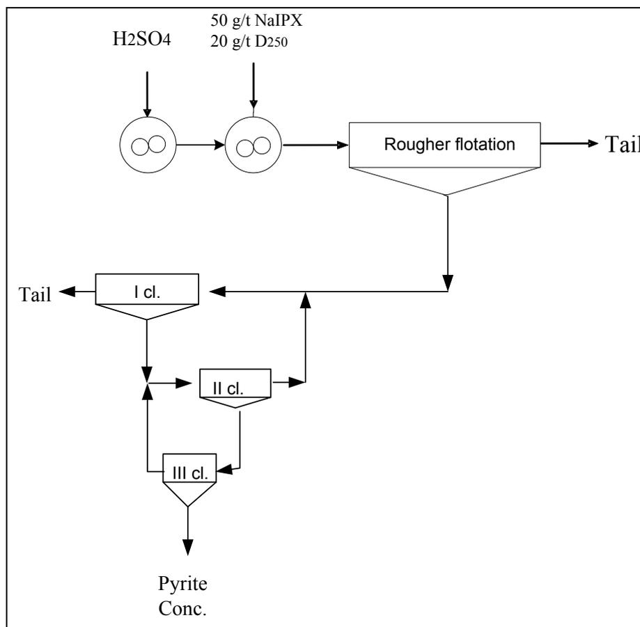
FIGURE 91 - FLOWSHEET FOR PRODUCTION PYRITE CONCENTRATE.
