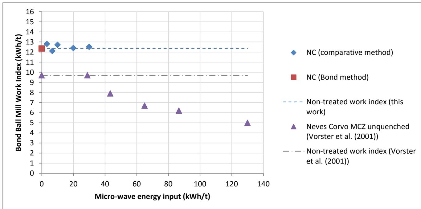
FIGURE 29 – BOND BALL MILL WORK INDEXES OF NEVES CORVO MICROWAVE TREATED AND UNTREATED SAMPLES: COMPARISON WITH THE WORK FROM VORSTER ET AL. (2001).
