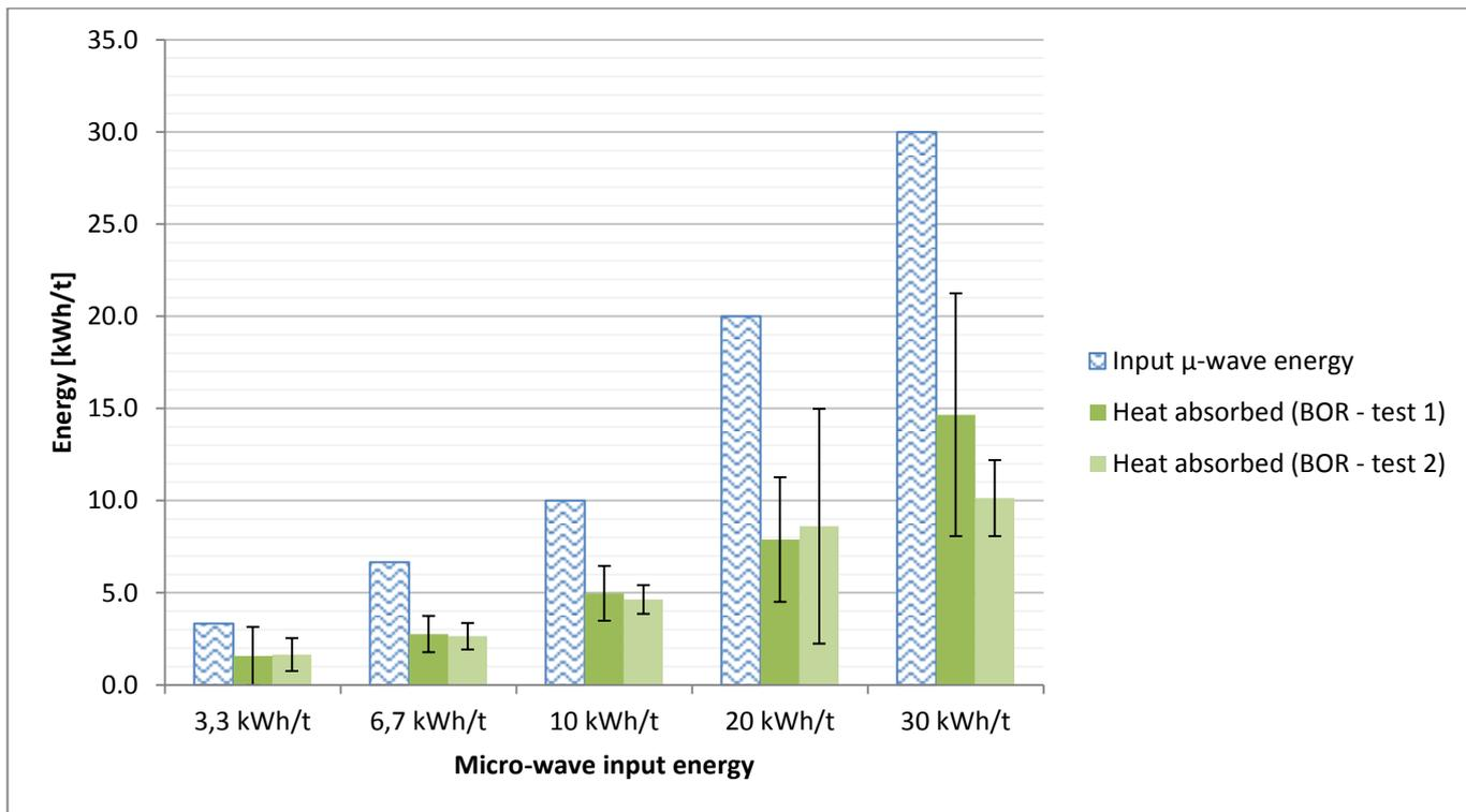
FIGURE 18 - CHART OF INPUT MICROWAVE ENERGY AND HEAT ABSORBED BY BOR SAMPLES.
