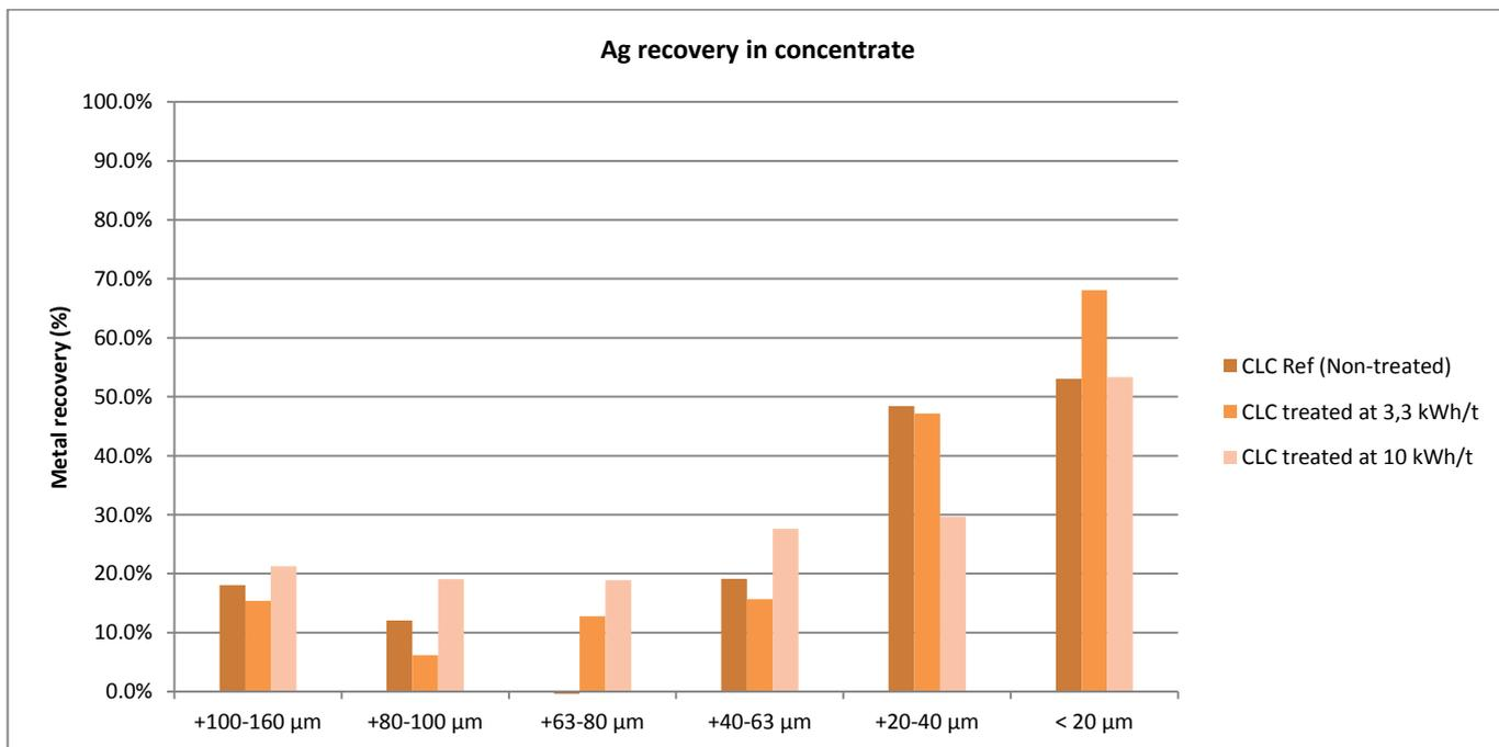
FIGURE 90 - AG RECOVERY PER SIZE FRACTION IN FLOTATION CONCENTRATE OF CLC TREATED AND UNTREATED SAMPLES.
