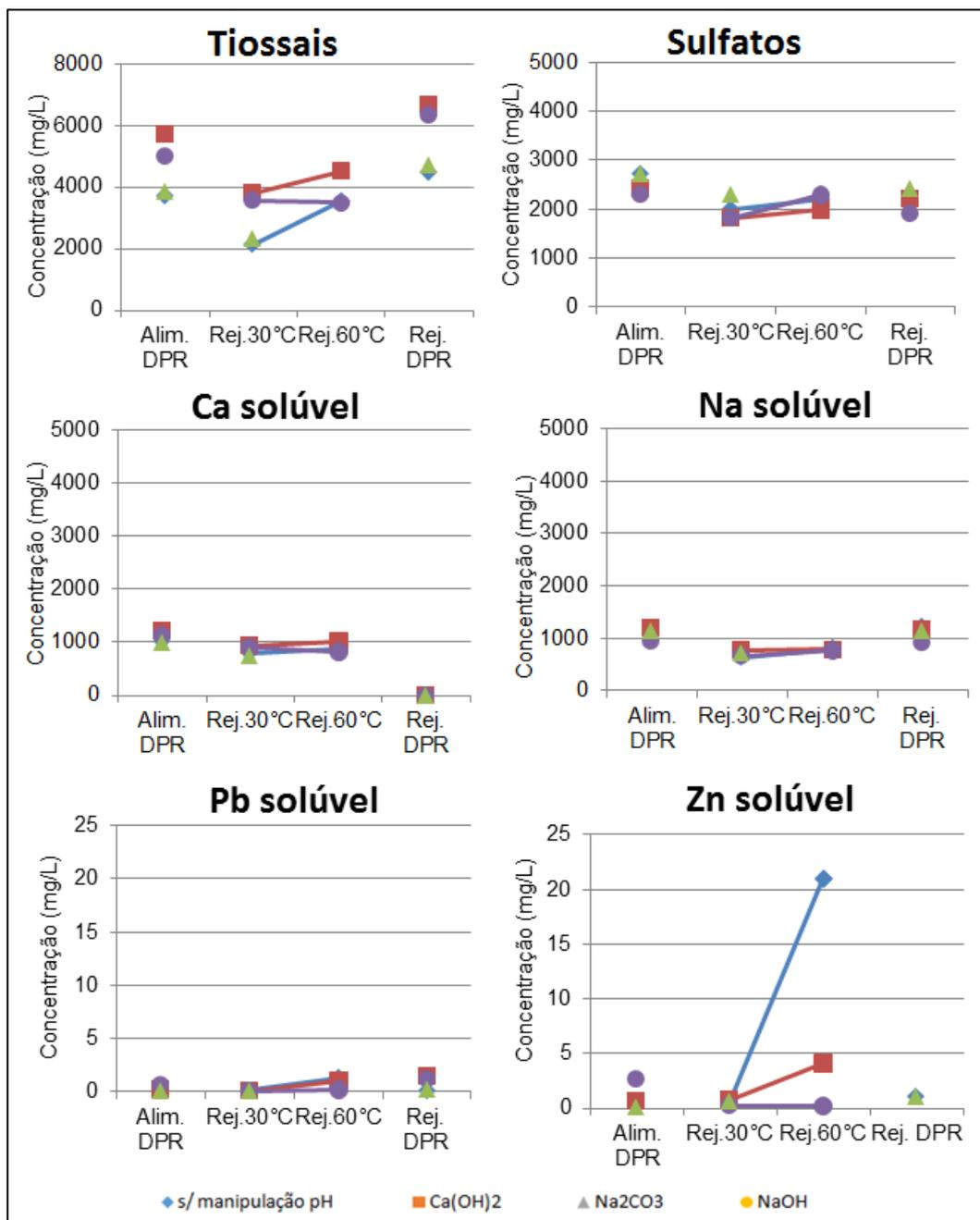
FIGURE 60 - CONCENTRATION OF VARIOUS ELEMENTS IN THE WASTE WATER FROM THE FLOTATION TESTS.
