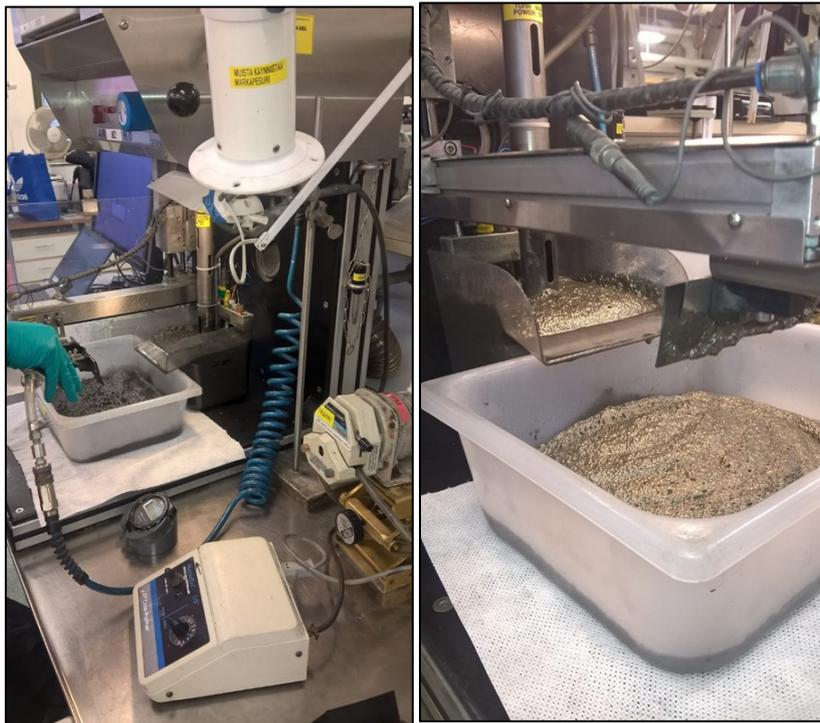
FIGURE 51 - INTMET WP2 BULK FLOTATION WITH GTK-OUTOTEC LABELL™.
