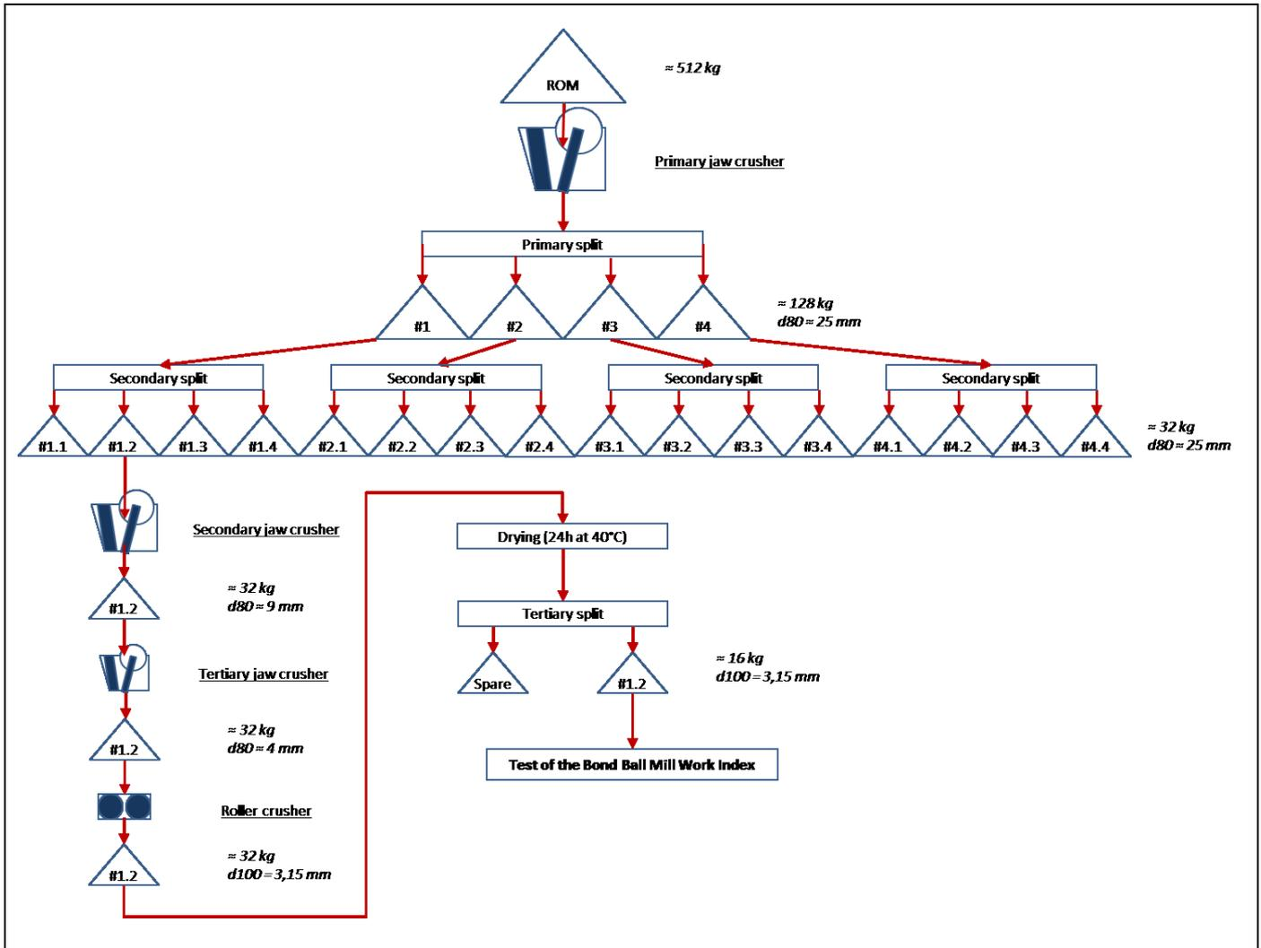
FIGURE 9 - SCHEME OF THE ORE PREPARATION DEDICATED TOWARDS BOND BALL MILL WORK INDEX DETERMINATION.
