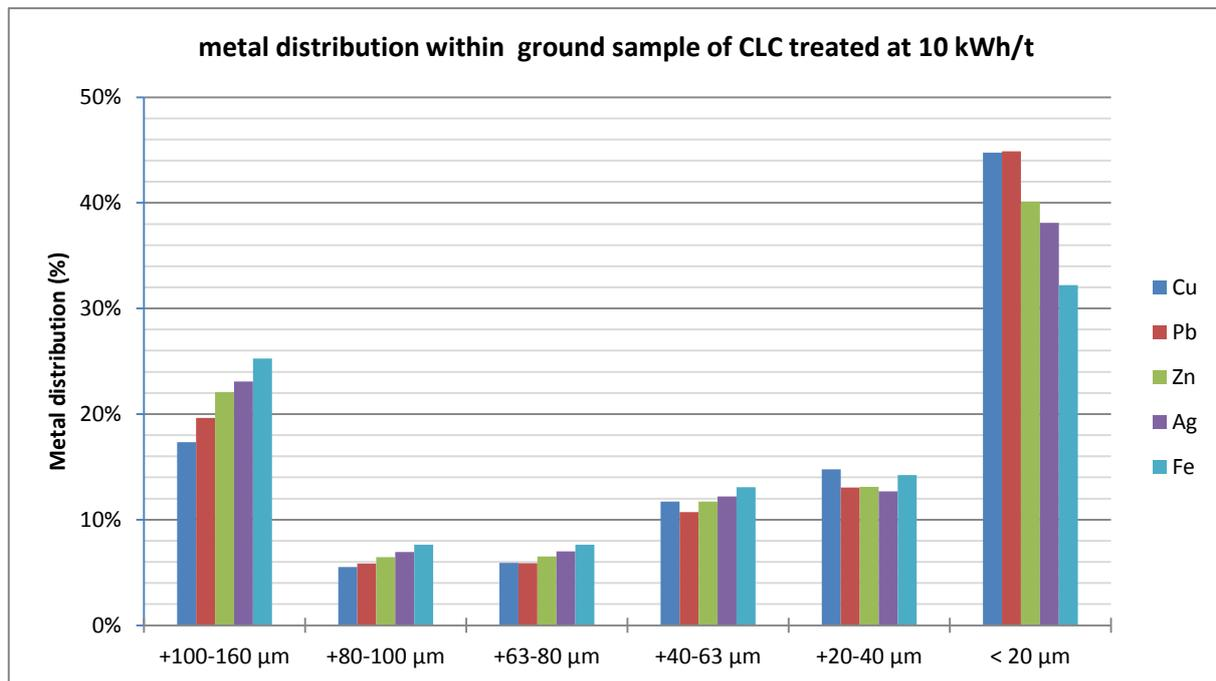
FIGURE 83 - METAL DISTRIBUTIONS BY SIZE FRACTION WITHIN GROUND SAMPLE OF CLC TREATED AT 10 KWH/T.
