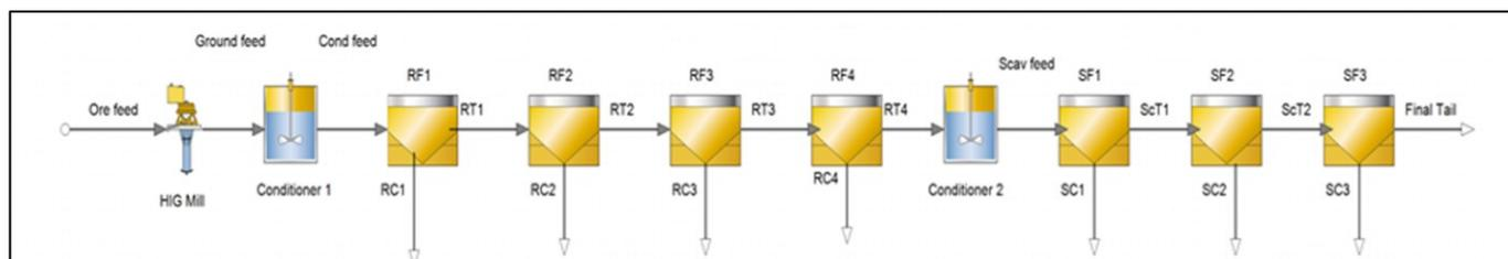
FIGURE 55 - PROCESS FLOW SHEET FOR HIGMILL TEST SERIES.
