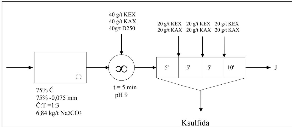
FIGURE 67 - SECOND EXPERIMENT SCHEME.
