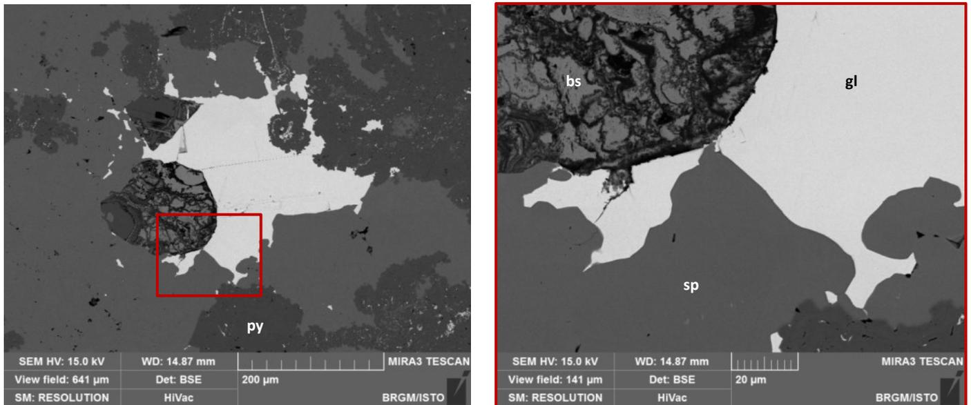
**FIGURE 21 - BSE PICTURES OF A CLC ORE SAMPLE TREATED AT 3.3 KWH/T (GL: GALENA; SP: SPHALERITE; PY: PYRITE; BS: BARYUM SULFATE).**
