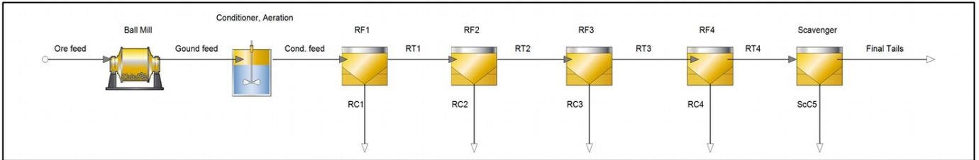
FIGURE 50 - PROCESS FLOWSHEET FOR BASELINE BULK FLOTATION WITH AERATION.
