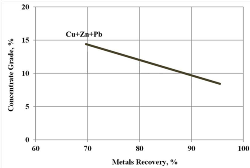
FIGURE 114 - RELATIONSHIP OF BULK CONCENTRATE OVERALL GRADE VS METALS RECOVERY.
