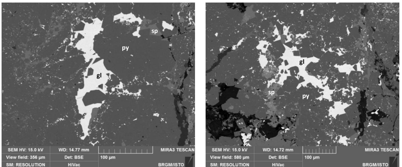
**FIGURE 22 - BSE PICTURES OF A NC ORE SAMPLE TREATED AT 30 KWH/T (GL: GALENA; SP: SPHALERITE; PY: PYRITE).**
