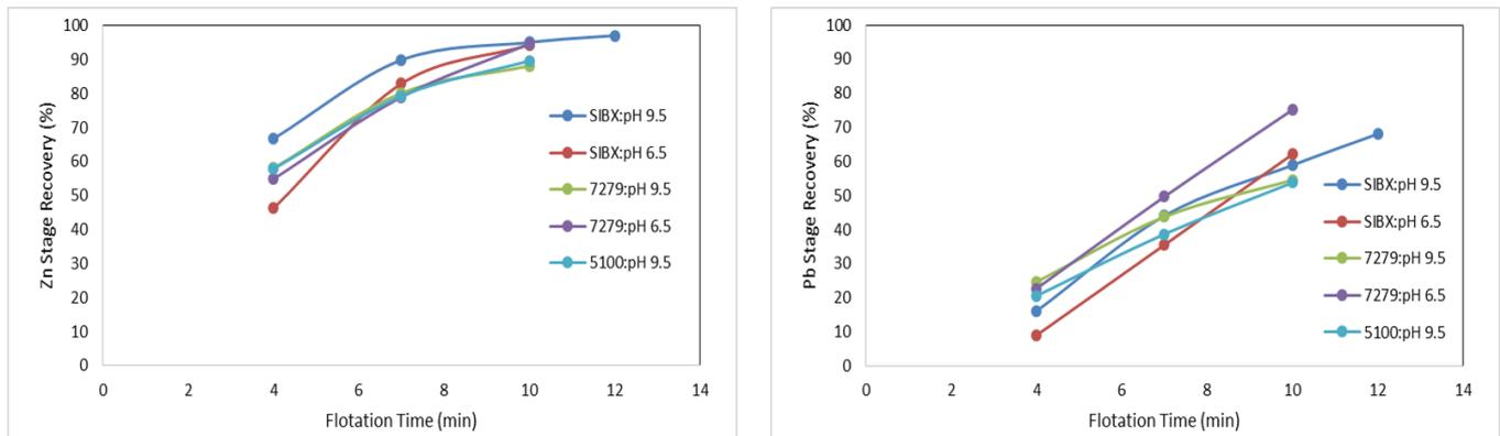
FIGURE 62 - STAGE RECOVERIES OF ZN AND PB AS FUNCTION OF FLOTATION TIME WITH DIFFERENT COLLECTOR TYPES AND PH.
