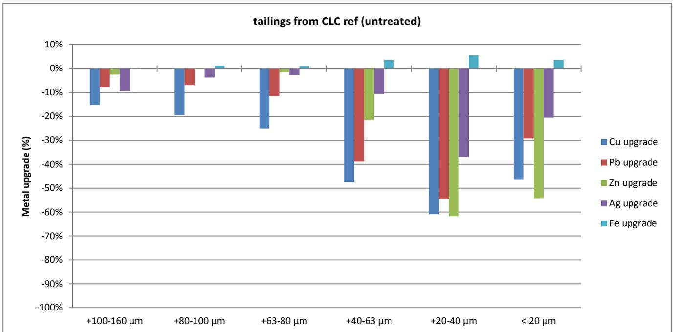
FIGURE 84 - METAL UPGRADE WITHIN THE TAILINGS OF THE FLOTATION TRIAL FROM CLC UNTREATED SAMPLE.
