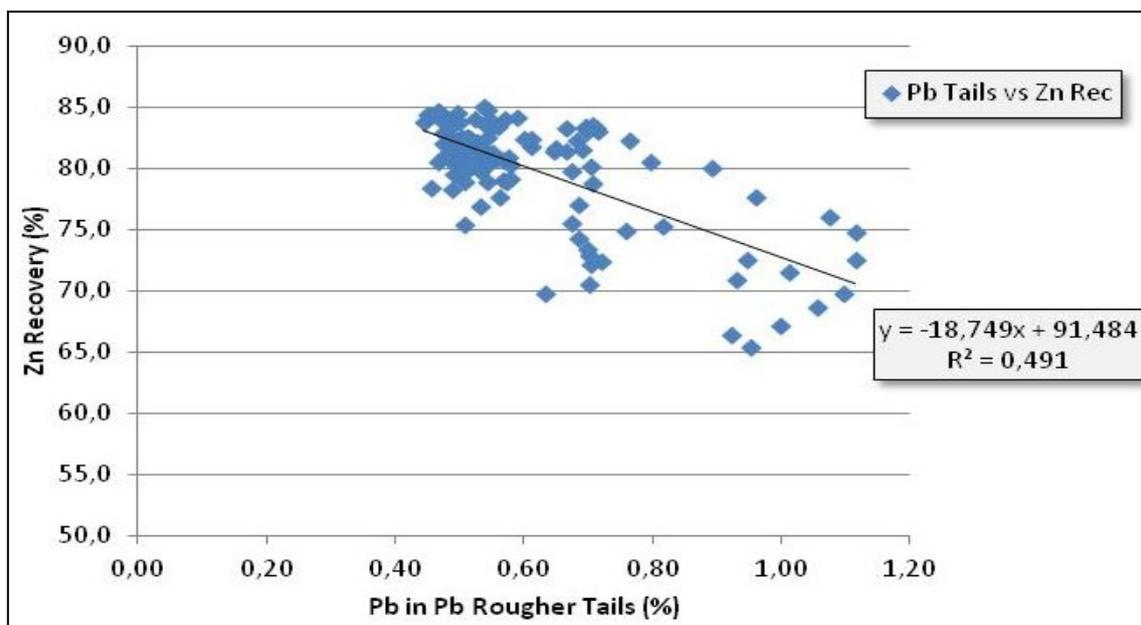
FIGURE 58 - EFFECT OF LEAD IN ZINC ROUGHER FEED ON MAIN ZINC CIRCUIT RECOVERY.
