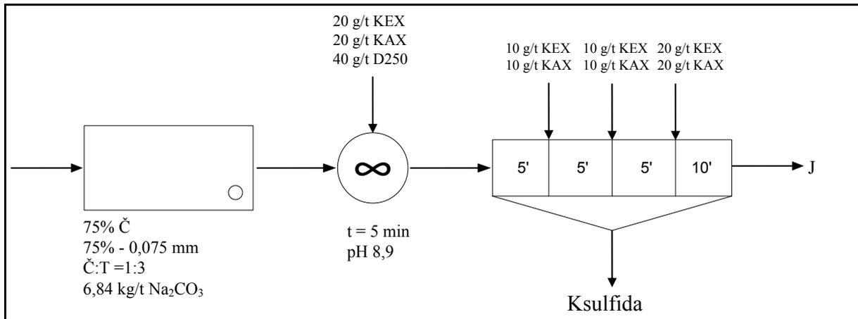
FIGURE 66 - FIRST EXPERIMENT SCHEME.
