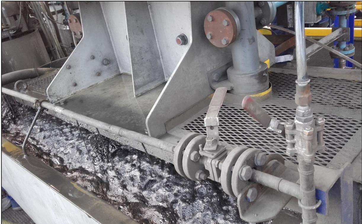
FIGURE 109 - CONCENTRATE PRODUCED IN A PILOT PLANT FLOTATION CELL.
