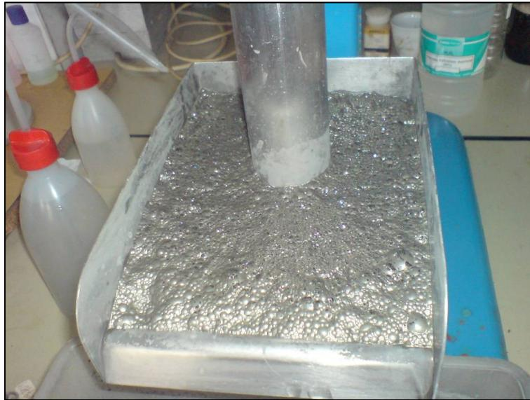
FIGURE 69 - SULPHIDE FLOTATION.
