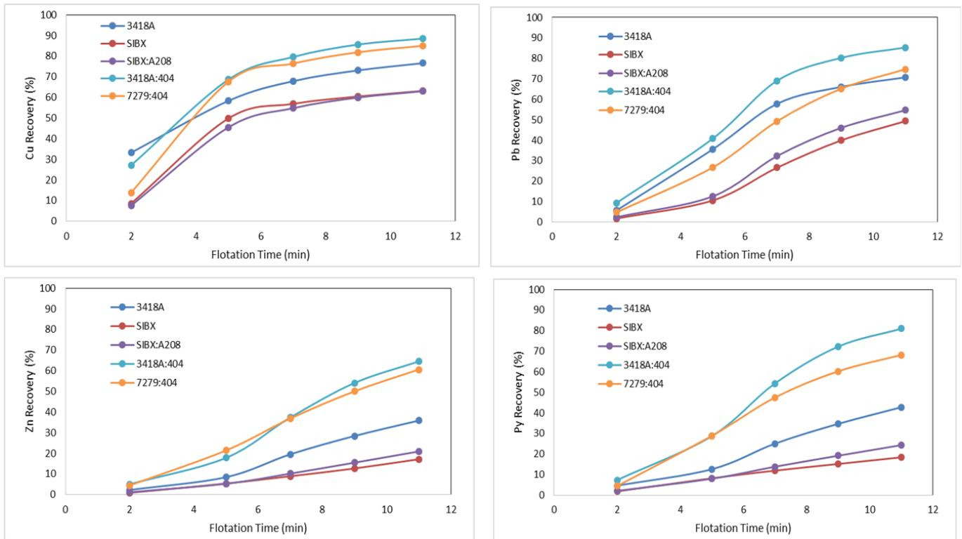
**FIGURE 61 - FLOTATION KINETICS OF THE SULPHIDE MINERALS WITH DIFFERENT COLLECTOR TYPES.**
