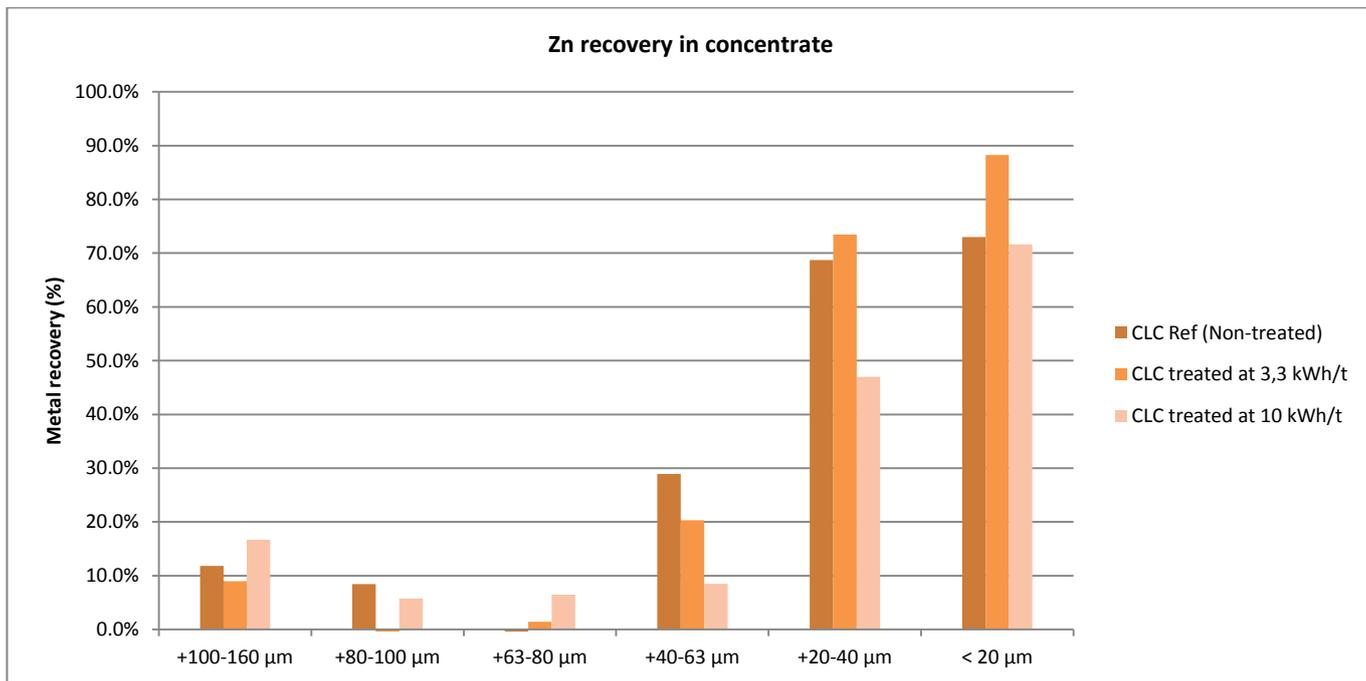
FIGURE 89 - ZN RECOVERY PER SIZE FRACTION IN FLOTATION CONCENTRATE OF CLC TREATED AND UNTREATED SAMPLES.
