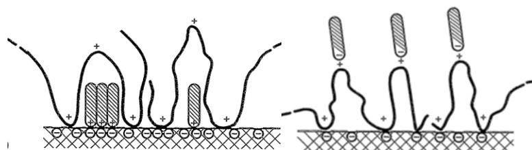
**FIGURE 30 - CO- ADSORPTION ON MINERAL PARTICLES RESULTING IN FLOTATION DEPRESSION AND FLOTATION ACTIVATION.**
