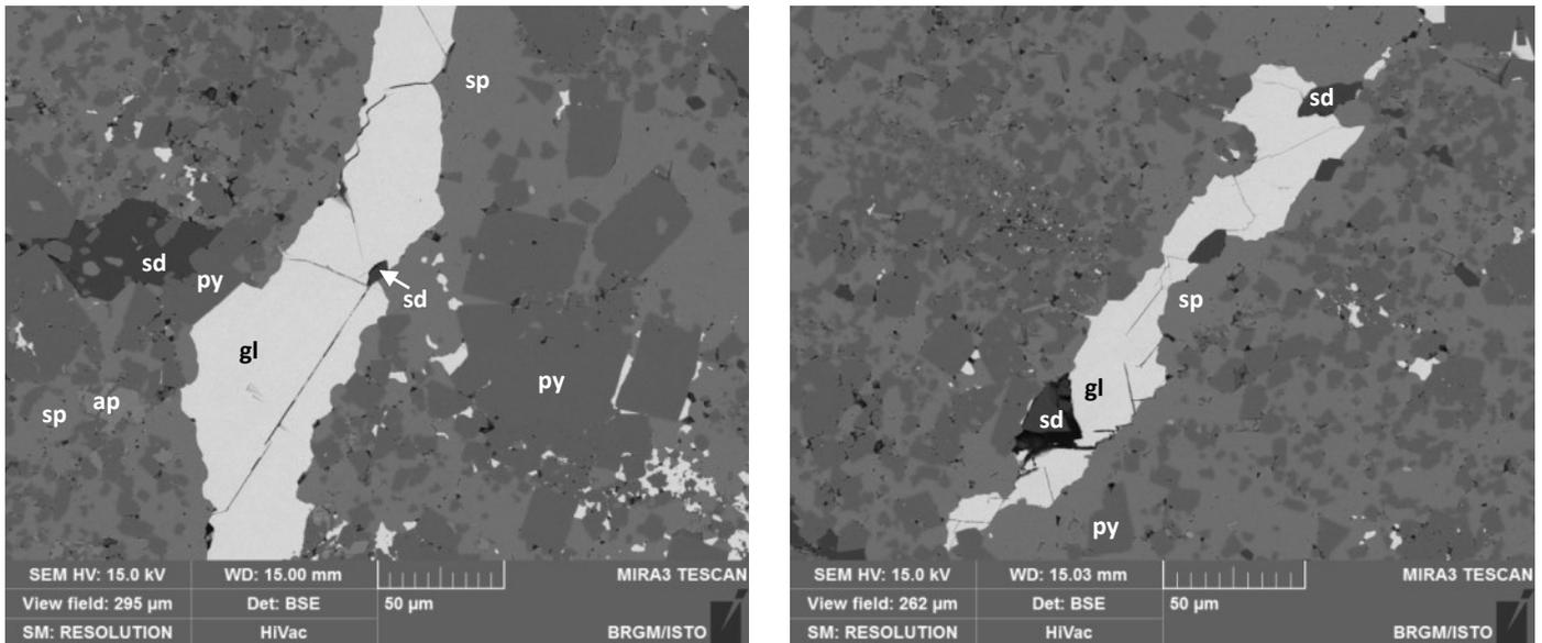
**FIGURE 23 - BSE PICTURES OF A NC ORE SAMPLE TREATED AT 30 KWH/T WITH INTRAGRANULAR FRACTURES OF GALENA (GL: GALENA; SP: SPHALERITE; PY: PYRITE; SD: SIDERITE; AP: ARSENOPYRITE).**
