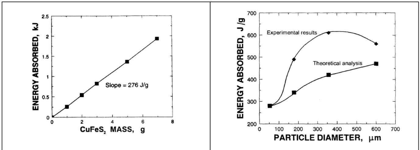
FIGURE 3 - [LEFT] ENERGY ABSORBED IN A QUARTZ/CHALCOPYRITE MIXTURE AS A FUNCTION OF WEIGHT PERCENT OF CHALCOPYRITE [RIGHT] MICROWAVE ENERGY ABSORBED PER GRAM OF CHALCOPYRITE AS A FUNCTION OF PARTICLE SIZE (EXTRACTED FROM SALSAMAN ET AL. 1996).
