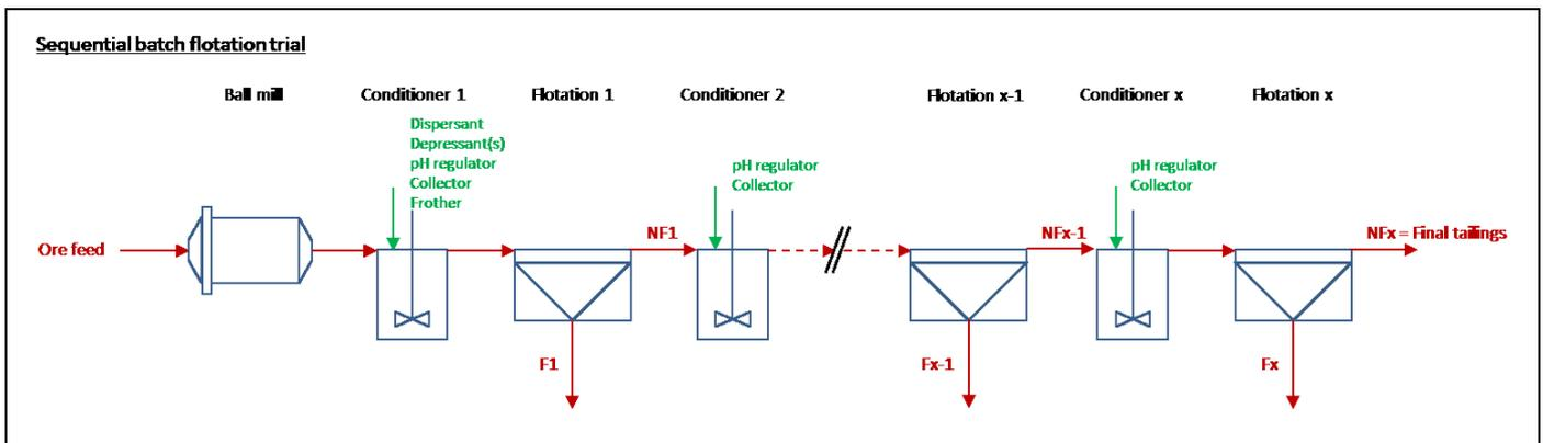
FIGURE 78 - PROCEDURE APPLIED FOR FLOTATION TRIALS.
