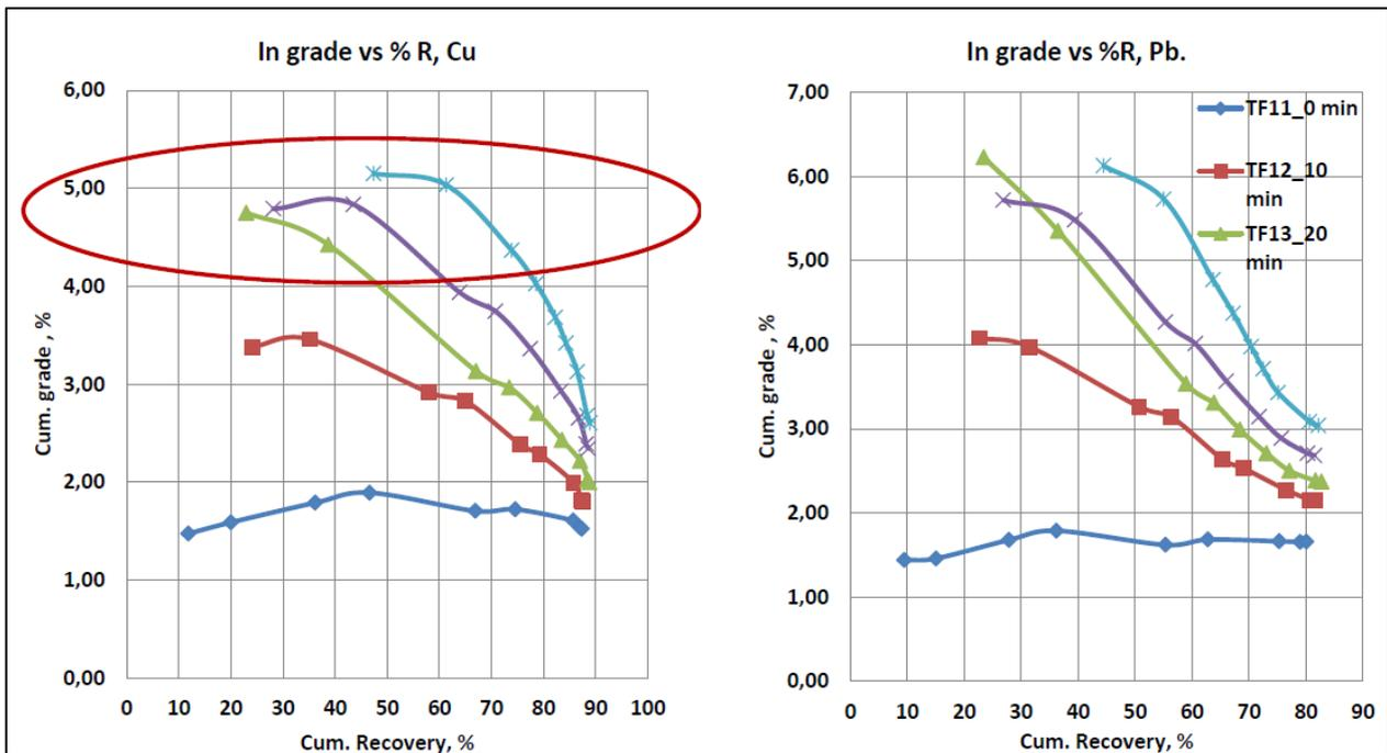
FIGURE 40 - COPPER AND LEAD RECOVERY VS PRE-AERATION TIME.
