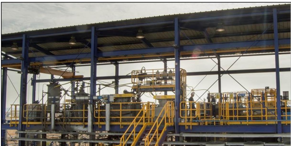
FIGURE 105 - CLC FLOTATION PILOT PLANT. GENERAL VIEW OF THE FLOTATION CELLS.
