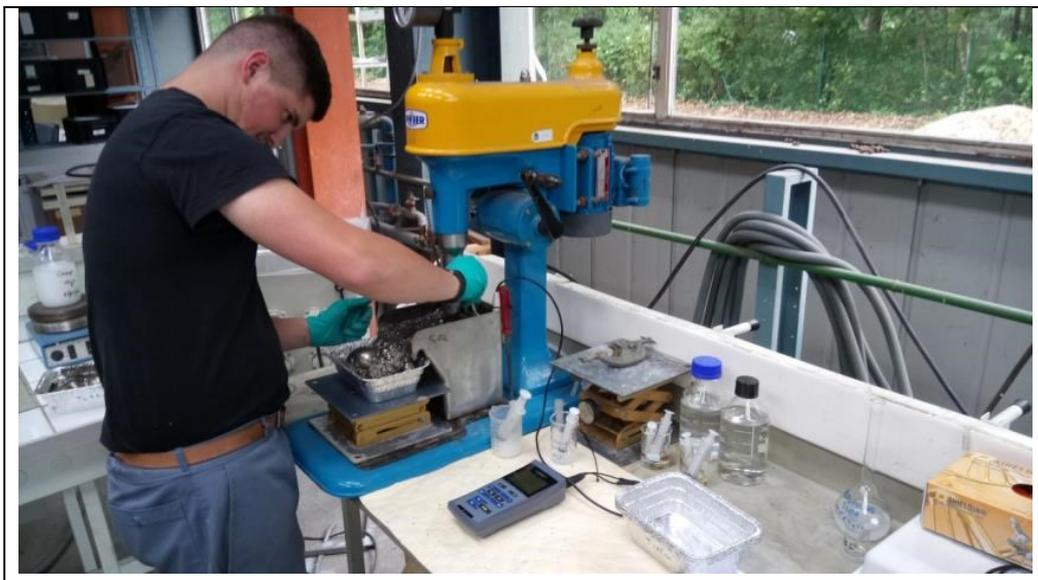
FIGURE 77 - FLOTATION TRIAL UNDER WAY WITH A 2,5L DENVER CELL.
