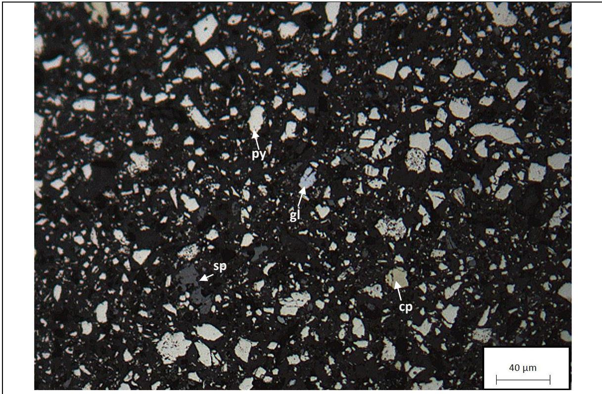
FIGURE 76 - PICTURES OF LIGHT TRANSMITTED MICROSCOPE OBSERVATION OF A MINUS 20 MICRONS FRACTION FROM A GROUND CLC SAMPLE (GL: GALENA; SP: SPHALERITE; PY: PYRITE; CP: CHALCOPYRITE).
