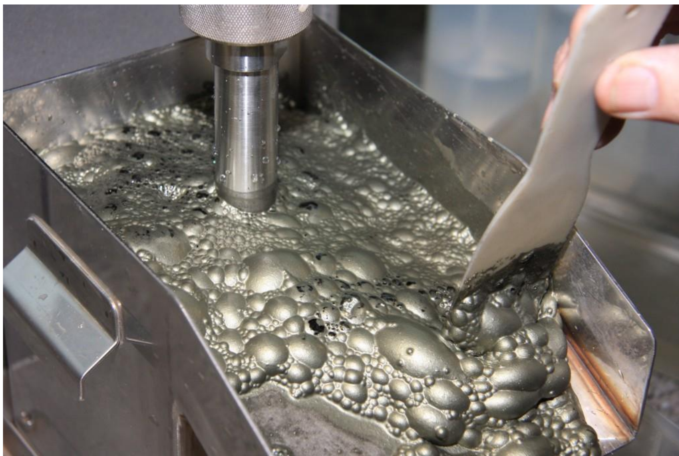
FIGURE 1. FLOTATION LAB CELL
