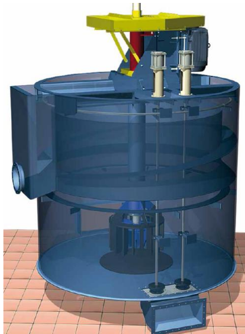
FIGURE 9. RCS FLOTATION MACHINE
