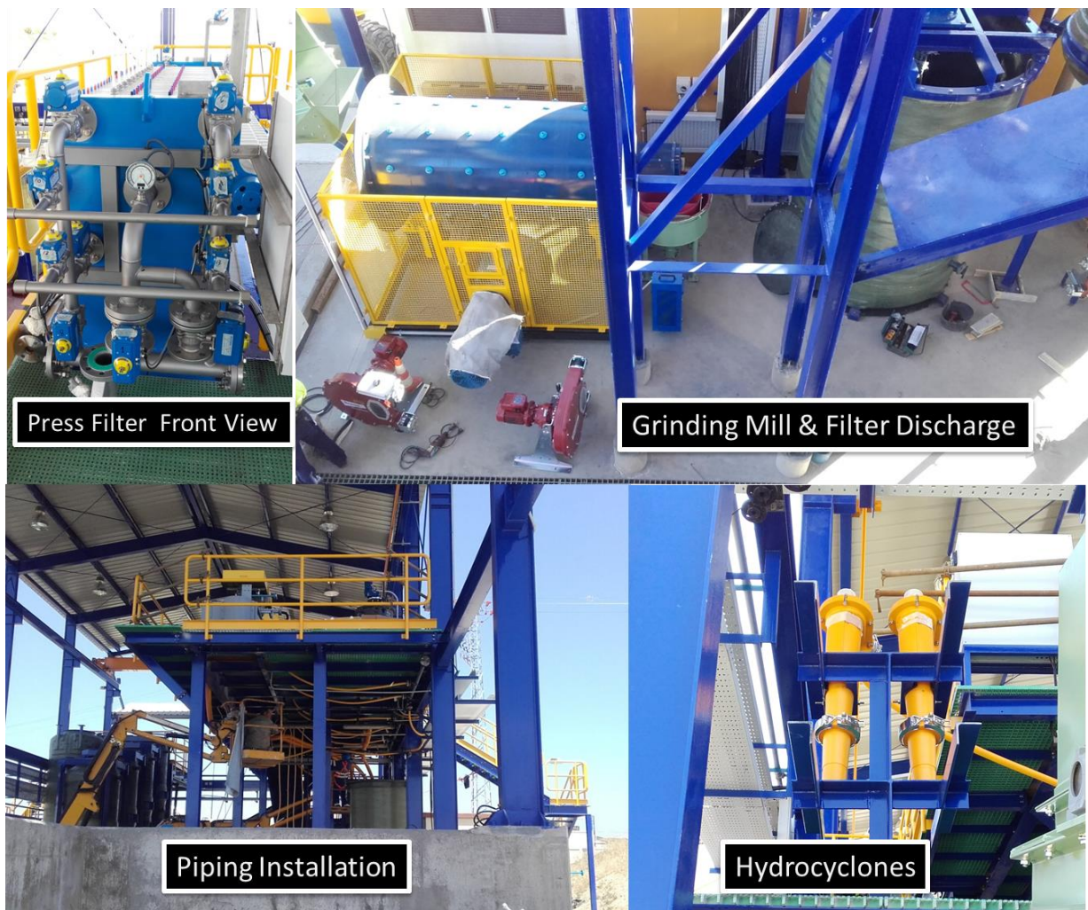
FIGURE 19. PILOT EQUIPMENT DETAILS
