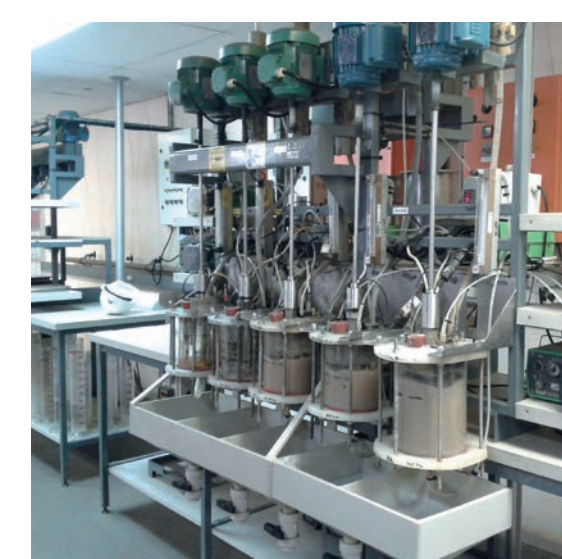
Continuous bioleaching at Mintek of the IRM-Bor, Somincor, KGHM (Lubin) and CLC feed materials
