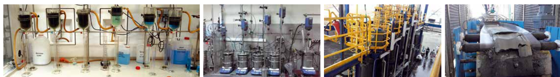
TR: Countercurrent test for copper SX at lab, CLC: Atmospheric leaching test at lab, CLC: Atmospheric leaching pilot plant design, commissioning, start up, running & fine tuning. PLS & leaching residue samples produced
