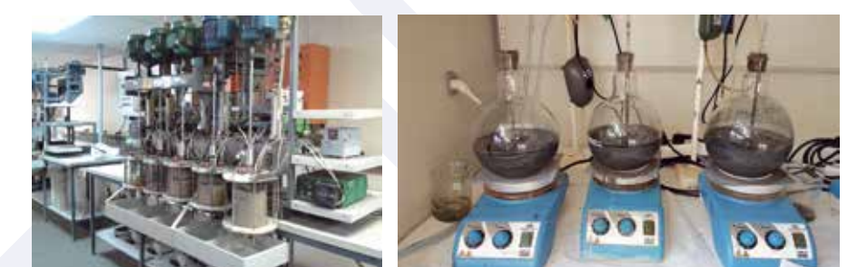
Continuous bioleaching at Mintek of the IRM-Bor, Somincor, KGHM (Lubin) and CLC feed materials, Cultivation of local bacterial cultures at BOR
