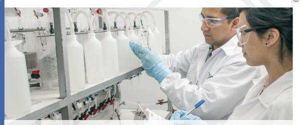
Humidity cell test. Soluble weathering products are mobilized by a fixed-volume aqueous leach that is performed and collected weekly. Leachate samples are analysed. © AGQ Mining and Bioenergy
