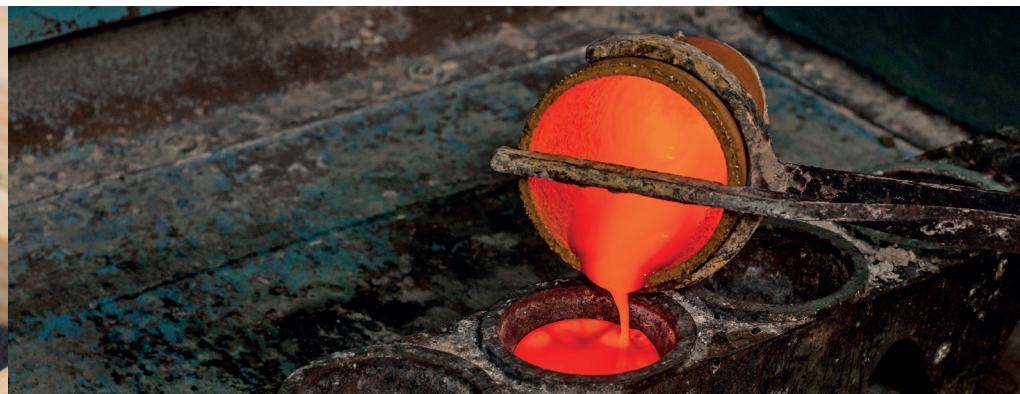
Fire assay is a classical method used for the separation of platinum group elements and gold by pre-concentration. After the fusion in a furnace, the mixture is poured into a mould for cooling. © AGQ Mining and Bioenergy
