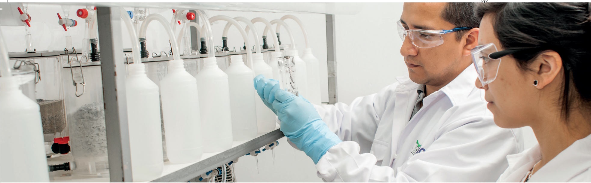
Humidity cell test. Temperature and humidity conditions of the cells are controlled and monitored during the test. © AGQ Mining and Bioenergy
